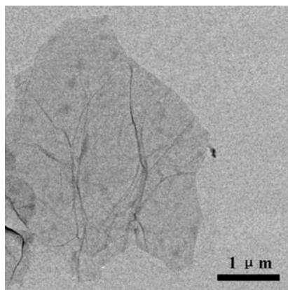
**Fig. S1** Typical TEM image of N-graphene
