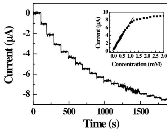
**Fig. S4** Typical steady state current response of the electrocatalytic reduction of H<sub>2</sub>O<sub>2</sub> by N-graphene on successive addition of 0.1 mM H<sub>2</sub>O<sub>2</sub> in solution (PBS, pH 7.4) under a constant potential of -400 mV. Inset shows the calibration curve of the electrocatalytic current on the concentration of H<sub>2</sub>O<sub>2</sub>.
