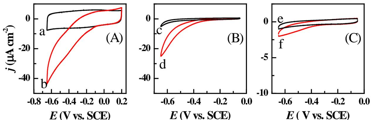
**Fig. S3** Voltammetric response of electrocatalytic reduction of 0.2 mM  $\text{H}_2\text{O}_2$  by N-graphene (A), N-free graphene (B), and bare GC (C). The responses were recorded in  $\text{N}_2$ -saturated PBS (0.1 M, pH 7.4) with (curves b, d, and f) and without (curves a, c, and e) of 0.2 mM  $\text{H}_2\text{O}_2$ . Scan rate was 100 mV/s.
