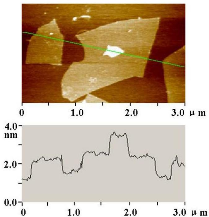
**Fig. S2** Typical AFM image of N-graphene
