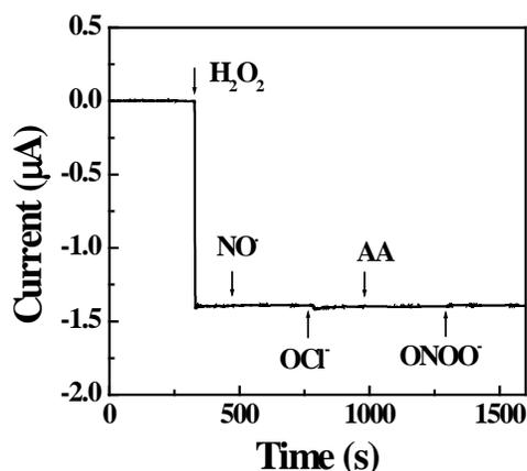
**Fig. S5** Amperometric response of  $\text{H}_2\text{O}_2$  (0.1 mM),  $\text{NO}^\cdot$  (0.1 mM), AA (0.1 mM),  $\text{OCl}^-$  (0.1 mM), and  $\text{ONOO}^-$  (0.1 mM) at the N-graphene/GC electrode under an applied potential of  $-400$  mV (versus SCE).
