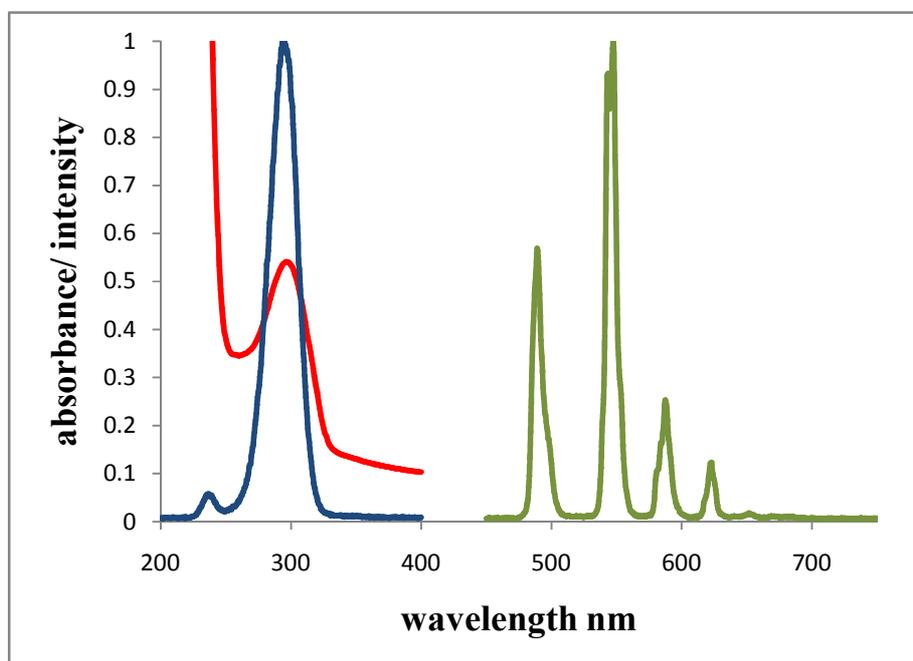
**Figure S2.** Absorbance (red) and normalized excitation (blue) and emission (green) spectra of  $\text{TbL}^2$  ( $\text{H}_2\text{O}$ , MOPS, pH 7.4).
