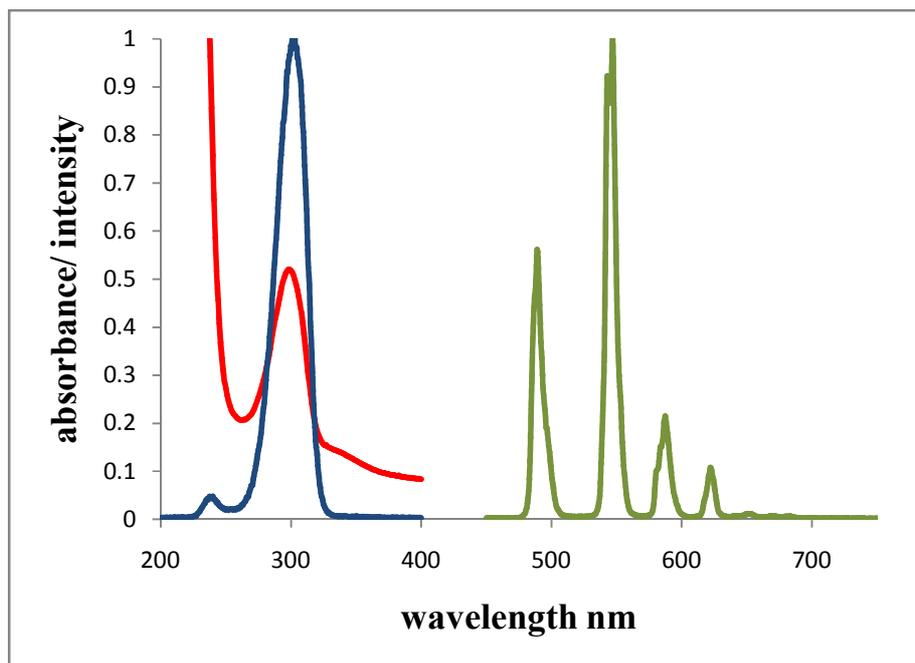
**Figure S3.** Absorption (red) and normalized excitation (blue) and emission (green) spectra of  $\text{TbL}^3$  ( $\text{H}_2\text{O}$ , MOPS, pH 7.4).
