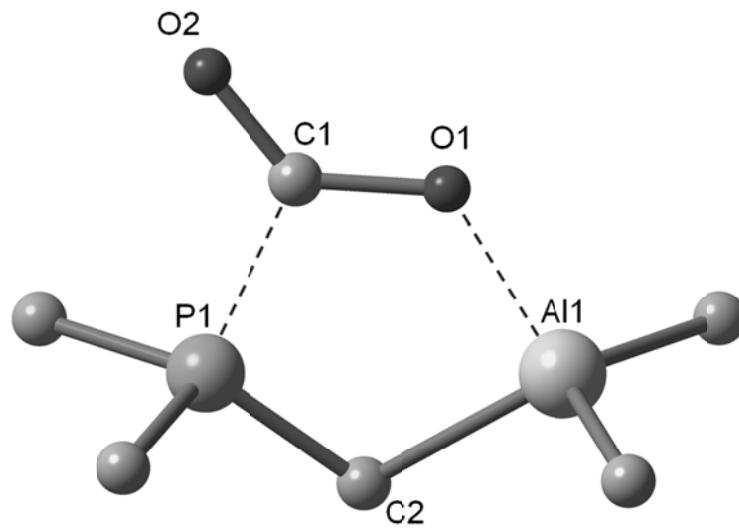
Selected bond lengths [Å] and angles [°]: P1-C1 1.907, C1-O1 1.288, C1-O2 1.216, O1-Al1 1.902, Al1-C2 2.110, P1-C2 1.771, O1-C1-O2 130.76, P1-C1-O2 118.08, C1-P1-C2 105.68, O1-Al1-C2 93.06.
