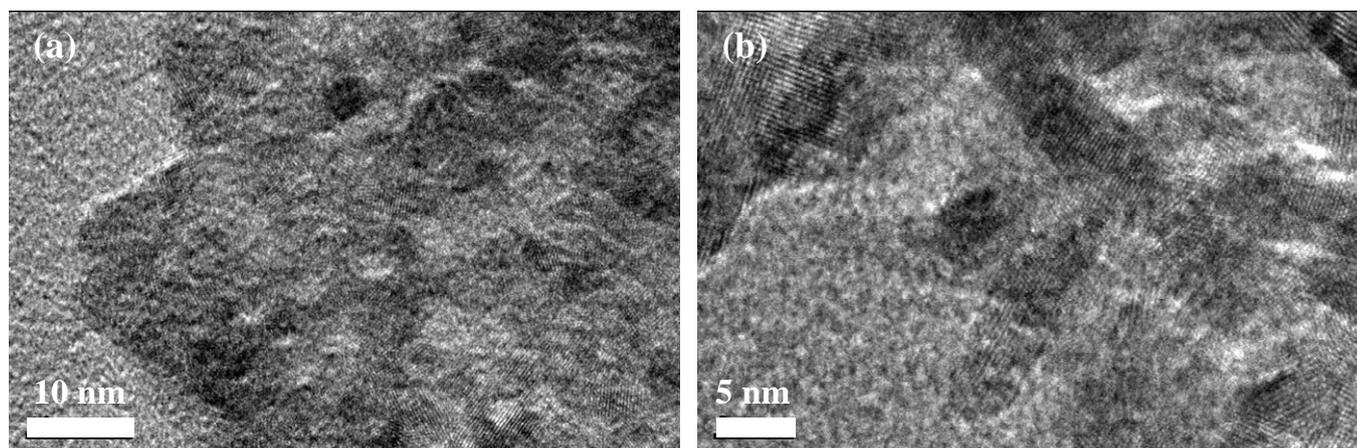
**Figure S2.** HR TEM images for (a) SnO<sub>2</sub> nanoparticles calcined at 250 °C and (b) SnO<sub>2</sub> nanoparticles calcined at 400 °C.
