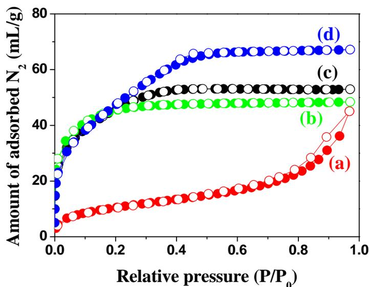
**Figure S3.** N<sub>2</sub> adsorption-desorption isotherms for (a) restacked titanate, (b) STN-I, (c) SnO<sub>2</sub> nanoparticles, and (d) STN-II. The filled and open symbols represent adsorption and desorption data, respectively.
