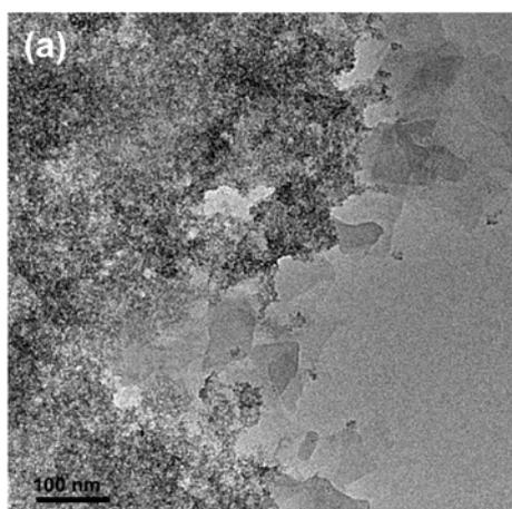
Fig. S2. TEM images of Pd/graphene composite synthesized without irradiant white-light
