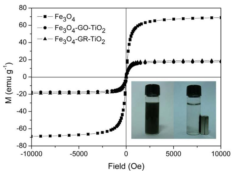
**Fig. S2** Room-temperature magnetization curves of  $\text{Fe}_3\text{O}_4$ ,  $\text{Fe}_3\text{O}_4\text{-GO-TiO}_2$  and  $\text{Fe}_3\text{O}_4\text{-GR-TiO}_2$ . Inset shows the magnetic response of  $\text{Fe}_3\text{O}_4\text{-GR-TiO}_2$  in the magnetic field generated from a magnet.
