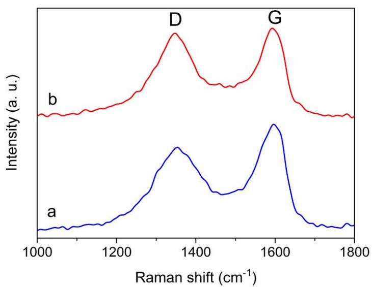
**Fig. S4** Raman spectra of Fe<sub>3</sub>O<sub>4</sub>-GO-TiO<sub>2</sub> (Intensity ratio  $I_D/I_G = 0.784$ ) (a) and Fe<sub>3</sub>O<sub>4</sub>-GR-TiO<sub>2</sub> ( $I_D/I_G = 0.944$ ) (b).
