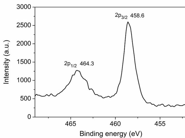
**Fig. S3** XPS spectra of Ti2p in the Fe<sub>3</sub>O<sub>4</sub>-GR-TiO<sub>2</sub> networks.
