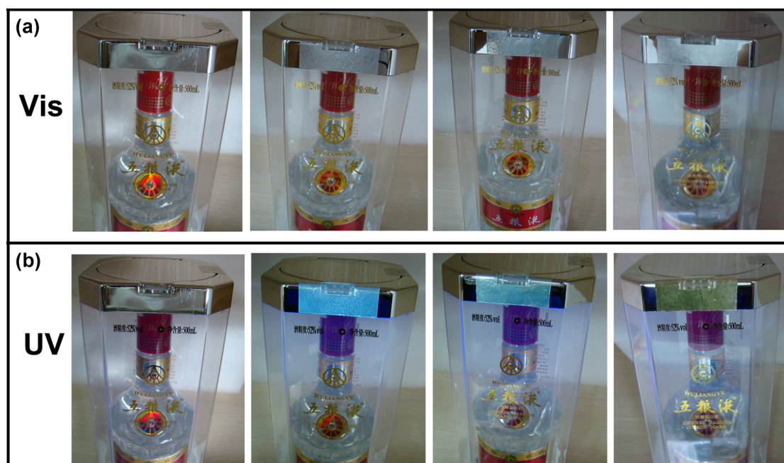
Figure S10. Digital photos of KH-560 modified ZnO QDs/PVA composite films for anti-counterfeit applications in expensive high-end liquors under (a) sunlight and (b) 302 nm UV light irradiation (from left to right: pure PVA film, film-B, film-D, and film-E). Obviously, the composite films emit visible lights with expected blue-yellow colors for anti-counterfeit purpose while the pure PVA film shows no emitting light under UV irradiation.
