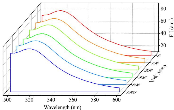
**Fig. S4** 3D waterfall of fluorescence spectra ( $\lambda_{\text{ex}} = 480$  nm) of fluorescein solution (10 nM) on addition of  $\text{AgNO}_3$ .
