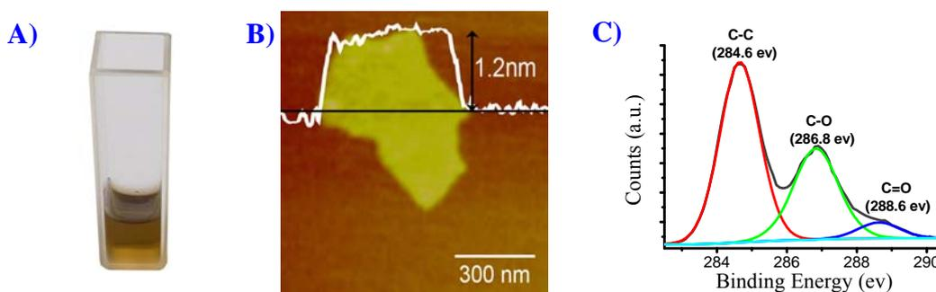
**Fig. S1.** A) Photograph of the as-prepared GO. B) AFM tapping-mode image of the as-prepared GO sheet. C) High-resolution XPS spectra of GO.
