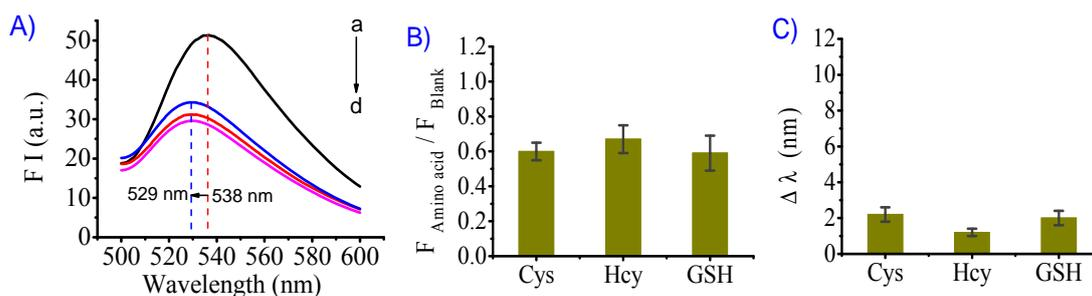
**Fig. S7** A) Fluorescence emission spectra of DNA1/DNA2/ $\text{Ag}^+$ /GO in the absence (a) and presence of Hcy (b), Cys (c), and GSH (d). B) The fluorescence intensity changes at fluorescence emission peak in the presence of Cys, Hcy, and GSH. C) The fluorescence emission wavelength changes relative to 528 nm in the presence of Cys, Hcy, and GSH. (DNA1/DNA2: 50 nM/50 nM,  $\text{Ag}^+$ : 1.5  $\mu$ M, Cys: 500 nM, Hcy: 500 nM, GSH: 500 nM, GO: 0.037 mg/mL,  $\lambda_{\text{ex}}$  = 480 nm).
