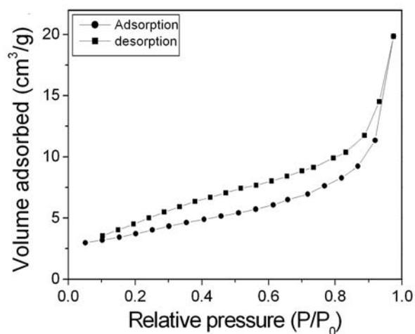
**Figure S3.** Nitrogen adsorption and desorption isotherms of the flowerlike  $\text{Co}_3\text{O}_4$  microspheres.
