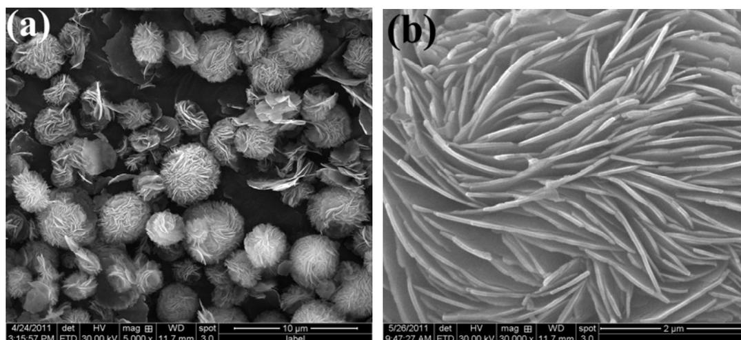
**Figure S1.** Representative SEM images of the  $\beta$ -Co(OH)<sub>2</sub> microspheres: (a) overall morphology of the products; (b) high-magnification SEM image of nanoplates in a microsphere.
