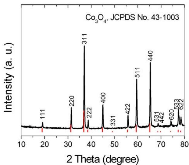
**Figure S9.** XRD patterns of the commercial  $\text{Co}_3\text{O}_4$  powder.
