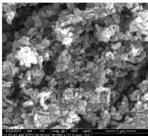
**Figure S8.** SEM image of the commercial  $\text{Co}_3\text{O}_4$  powder (JOHNSON MATTHEY Inc.).
