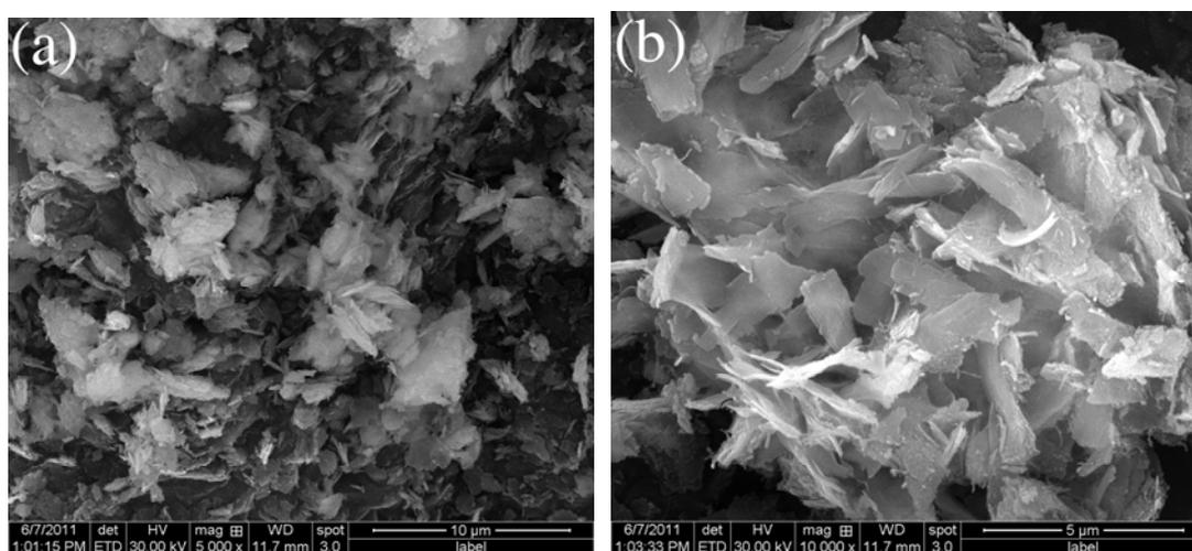
**Figure S7.** SEM images of the product obtained with ethanol in place of replace EG.
