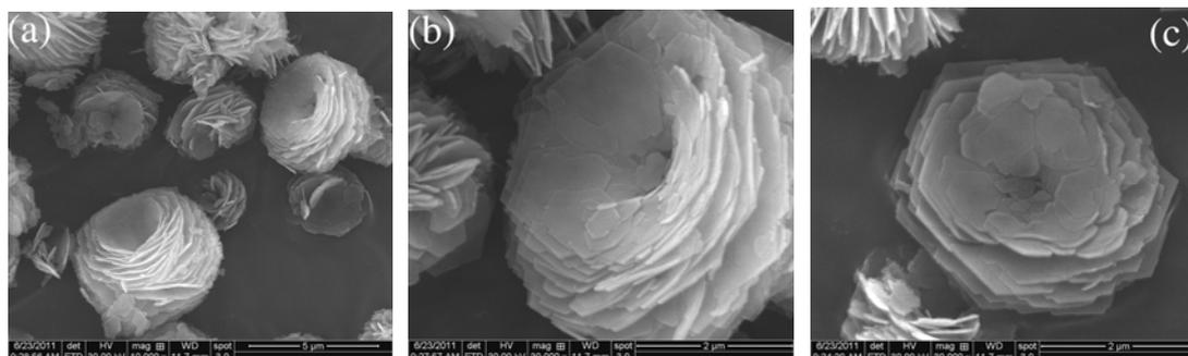
**Figure S4.** SEM images of the product obtained after hydrothermal reaction for 8 h, showing evidence of an assembly process of the microspheres via nanoplates.
