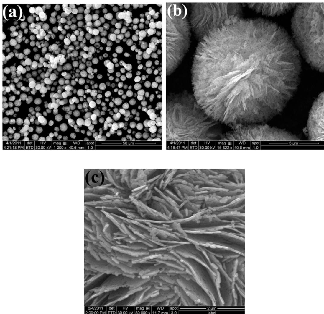
**Figure S2.** Representative SEM images of the  $\text{Co}_3\text{O}_4$  microspheres: (a) overall morphology of the products; (b) high-magnification SEM image of an individual microspheres; (c) high-magnification SEM image of nanoplates in a microsphere.
