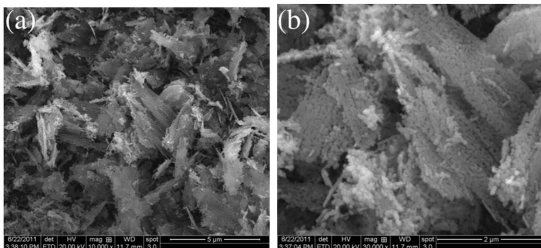
**Figure S6.** SEM images of the product consisting of nanocrystalline  $\text{Co}_3\text{O}_4$  obtained with twice the amount of  $\text{NH}_3 \cdot \text{H}_2\text{O}$  and calcining at  $400^\circ\text{C}$  for 4 h.
