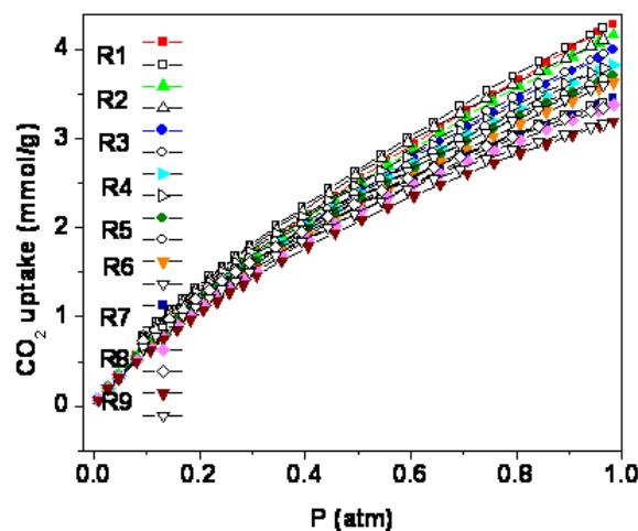
Figure S10. Cyclic adsorption of CO<sub>2</sub> for a-NDC6 at 298K via vacuum desorption.
