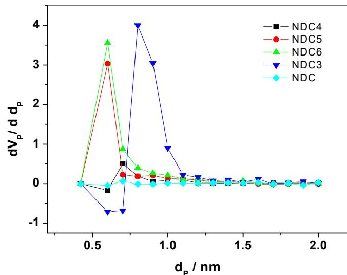
**Figure S8.** Pore volume distribution calculated by the MP method
