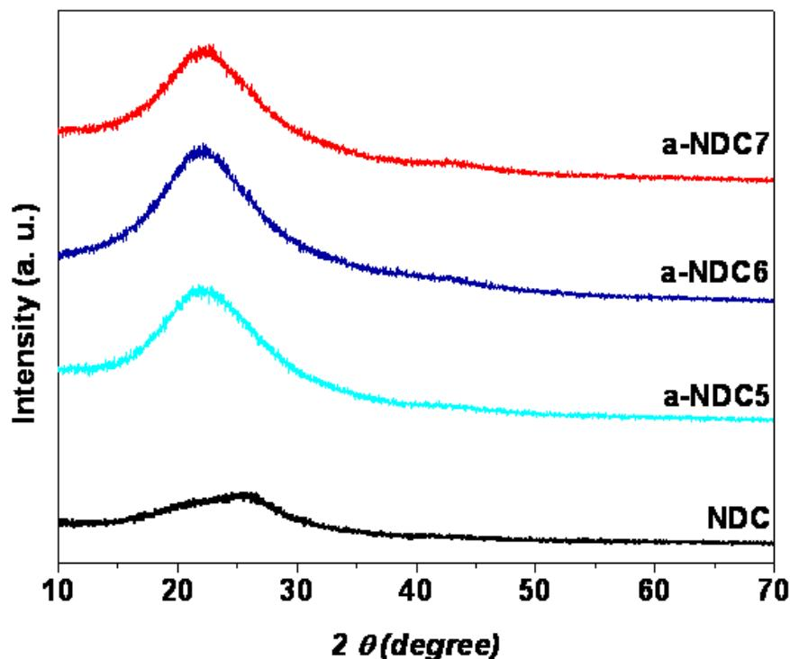
**Figure S3.** Powder X-ray diffraction pattern of adsorbents before and after chemical activation, showing the formation of amorphous phase.
