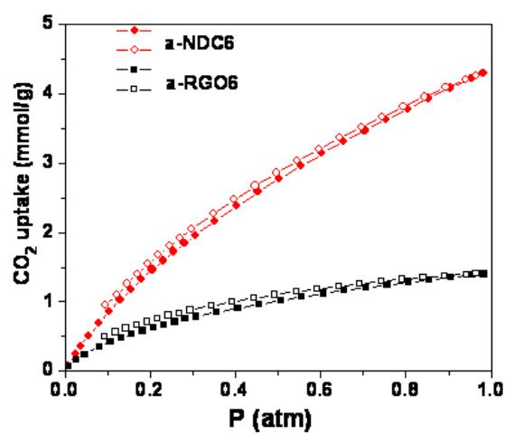
**Figure S9.** CO<sub>2</sub> adsorption isotherms for a-RGO6 and a-NDC6 at 298°K (filled symbols –adsorption and open symbols - desorption).
