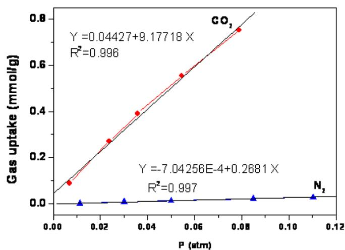
Figure S11. Initial slopes calculation from CO<sub>2</sub> and N<sub>2</sub> adsorption isotherms at 298K for a-NDC6.
