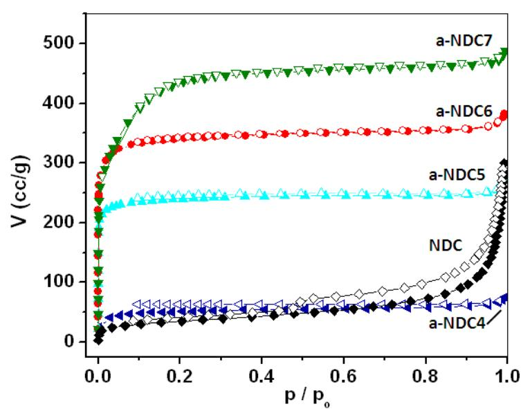
**Figure S7.**  $\text{N}_2$  adsorption – desorption for NDC and a- NDC.
