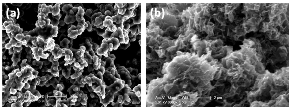
**Fig. S2.** SEM image of polypyrrole (a) and RGO (b).
