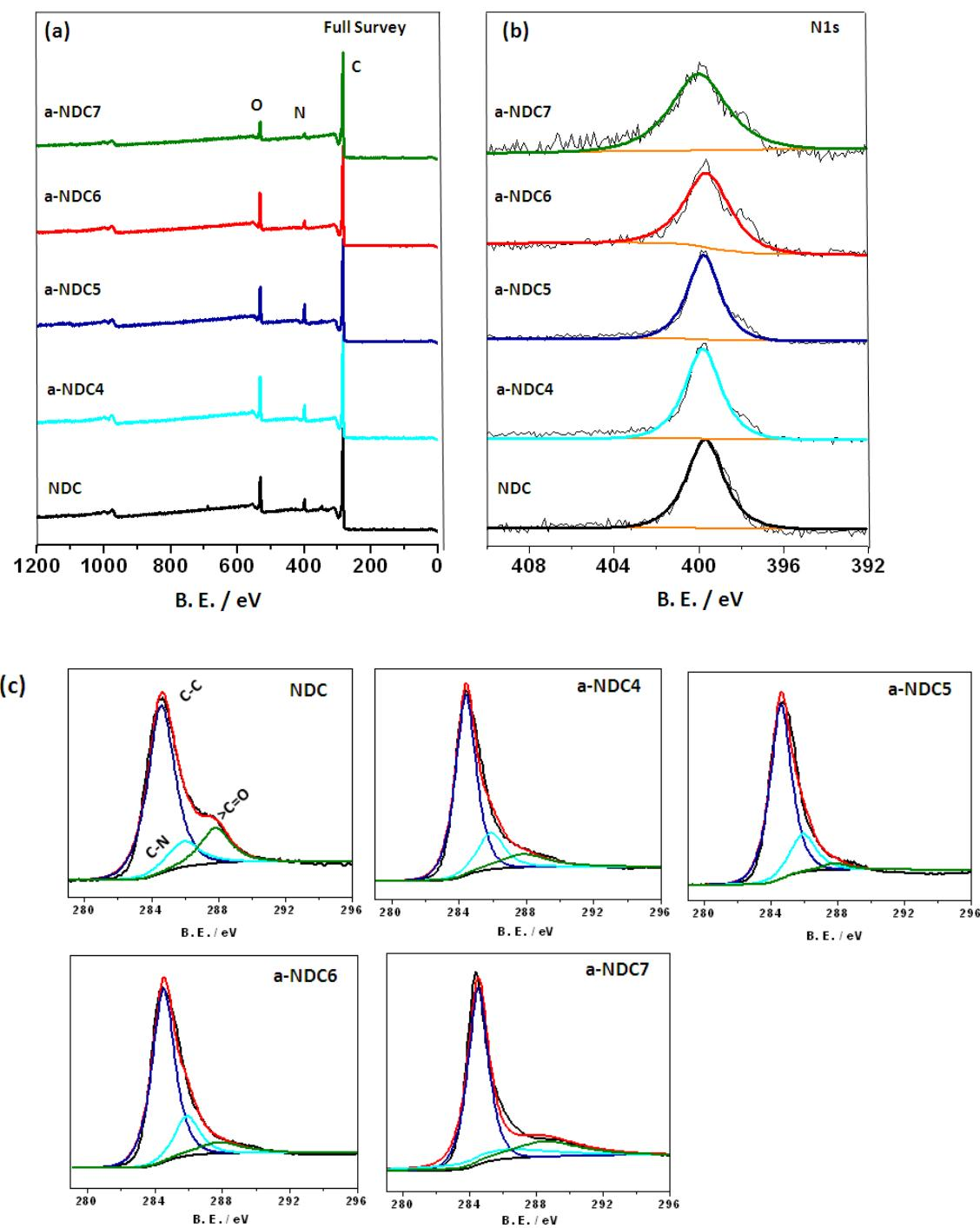
**Figure S6.** XPS spectra of adsorbents (a) Full Survey (b) Survey for N and (c) survey for C.
