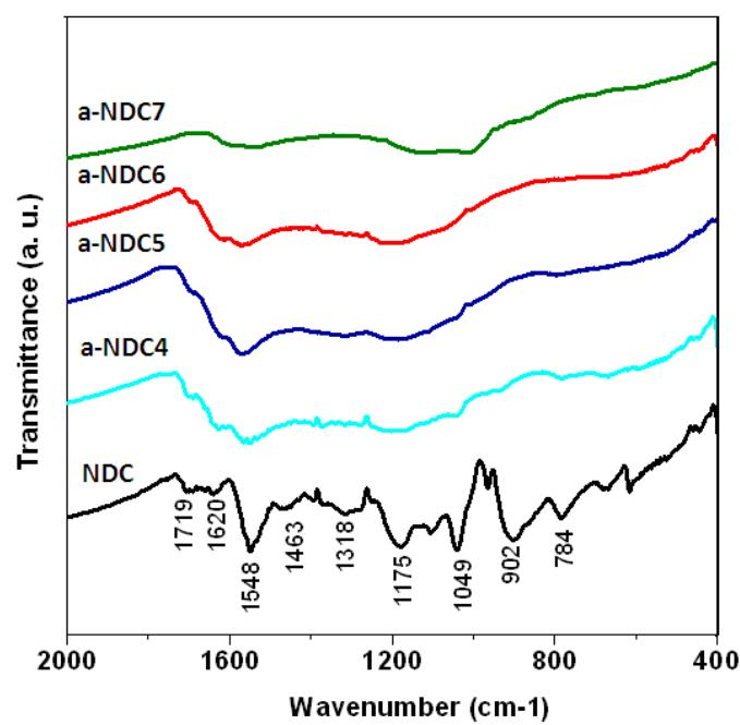
**Figure S5.** FTIR spectra of NDC and a-NDC (400, 500, 600 and 600 degree C).
