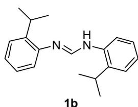
2-isopropylamine (2.0 g, 2.1 mL, 14.80 mmol, 2 eq.), triethylorthoformate (1.1 g, 1.2 mL, 7.40 mmol, 1 eq.) and glacial acetic acid (22.2 mg, 21  $\mu\text{L}$ , 0.37 mmol, 0.05 eq.) were mixed and stirred at 140 °C for 3 h. The crude solid was triturated in cold PE and filtered through a glassfrit. The solid was
