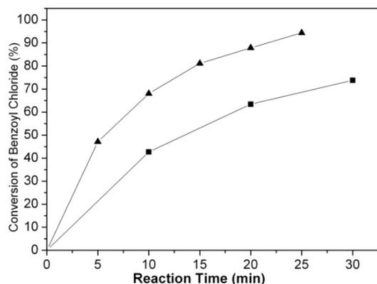
**Figure S5** Kinetic profiles of the Synthesis of benzoic anhydride. ■ blank test, ▲ catalyzed by 0.40 g PHCSs.
