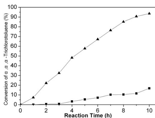
**Figure. S4** Kinetic profiles of the hydrolysis of  $\alpha,\alpha,\alpha$ -Trichlorotoluene. ■blank test, ▲ catalyzed by 0.40 g PHCSs.
