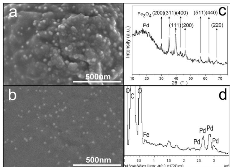
**Figure S9.** (a) SEM image of the magnetic Pd-PHCs. (b) BSE-SEM image of the magnetic Pd-PHCs. (c) XRD pattern of the magnetic Pd-PHCs. (d) Energy dispersive X-ray spectroscopy measurements of the magnetic Pd-PHCs.
