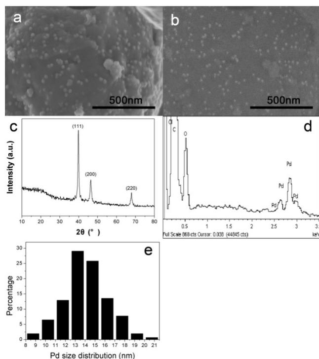
**Figure S6.** (a) SEM image of the Pd-PHCSs. (b) BSE-SEM image of the Pd-PHCSs. (c) XRD pattern of the Pd-PHCSs. (d) Energy dispersive X-ray spectroscopy measurements of Pd-PHCSs. (e) The size distribution of palladium nanoparticles on the Pd-PHCSs.
