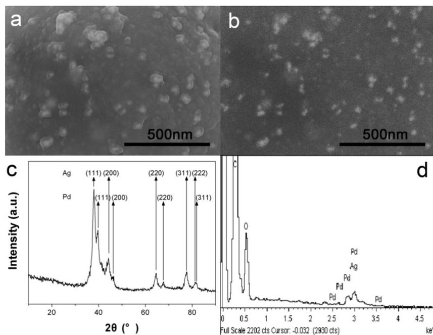
**Figure S8.** (a) SEM image of the Ag-Pd-PHCs. (b) BSE-SEM image of the Ag-Pd-PHCs. (c) XRD pattern of the Ag-Pd-PHCs. (d) Energy dispersive X-ray spectroscopy measurements of the Ag-Pd-PHCs.
