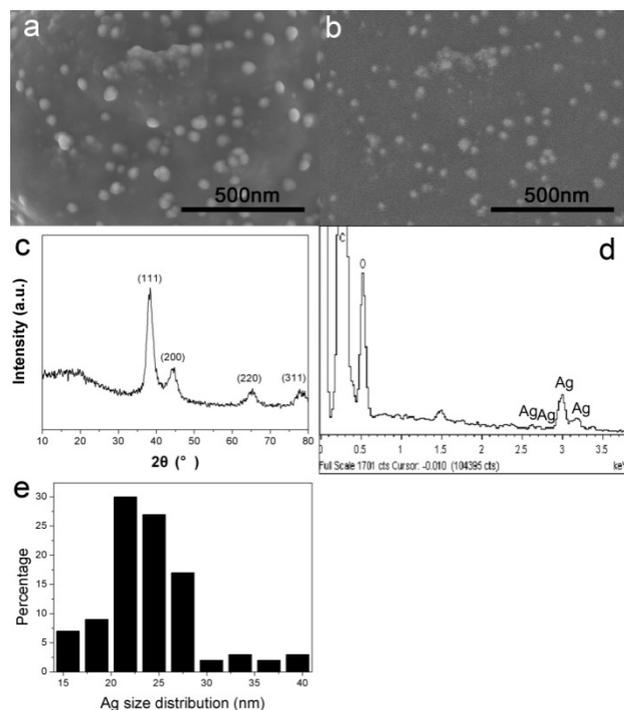
**Figure S7.** (a) SEM image of the Ag-PHCSs. (b) BSE-SEM image of the Ag-PHCSs. (c) XRD pattern of the Ag-PHCSs. (d) Energy dispersive X-ray spectroscopy measurements of Ag-PHCSs. (e) The size distribution of silver nanoparticles on the Ag-PHCSs.
