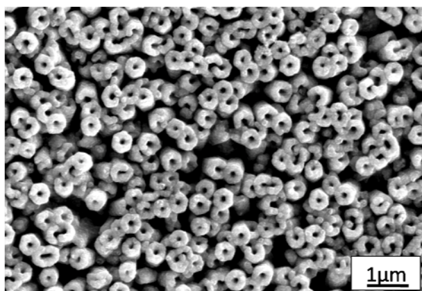
Figure S3 SEM image of the CdS/ZNT arrays after 30 min stability test at a fixed working electrode potential of 0 v vs SCE.
