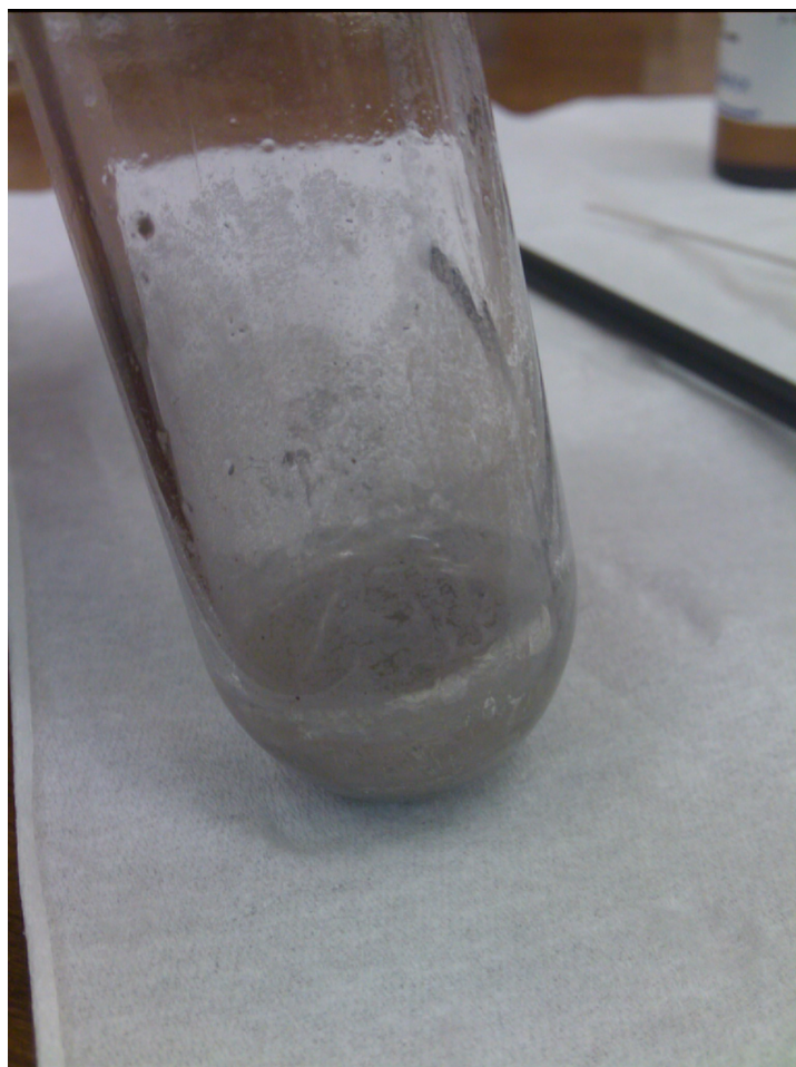
Figure 1: The dye sensitised ZnO/AgNO 3 /TEMPO system at the end of the reaction. The precipitated silver is evident on the sides of the reaction vessel. Reaction conditions: Benzyl alcohol (0.1 mmol) TEMPO (1.5 mg), dye sensitised ZnO (20 mg) and silver nitrate (18 equivalents) in 1.5 ml H 2 O under visible light irradiation for 2 hours.
