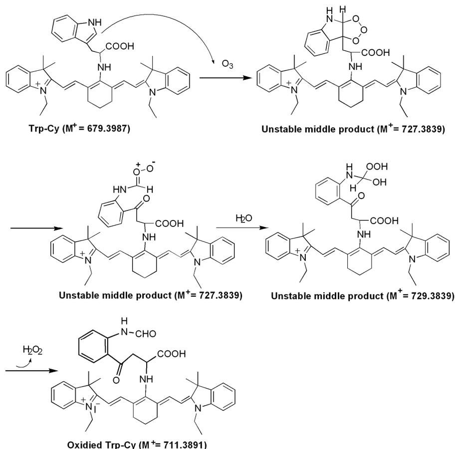
**Scheme S1.** A proposed molecular mechanism of Trp-Cy to recognize ozone
