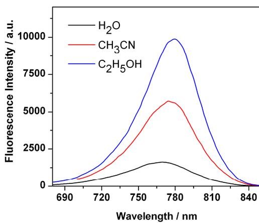
**Figure S1.** Fluorescence intensities of 10  $\mu$ M Trp-Cy dissolved in H<sub>2</sub>O, CH<sub>3</sub>CN and C<sub>2</sub>H<sub>5</sub>OH, respectively.
