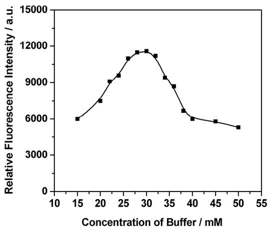
**Figure S3.** The relationship between the relative fluorescence intensity and concentration of the PBS buffer (10  $\mu\text{M}$  for Trp-Cy and 6  $\mu\text{M}$  for ozone, pH = 7.4)
