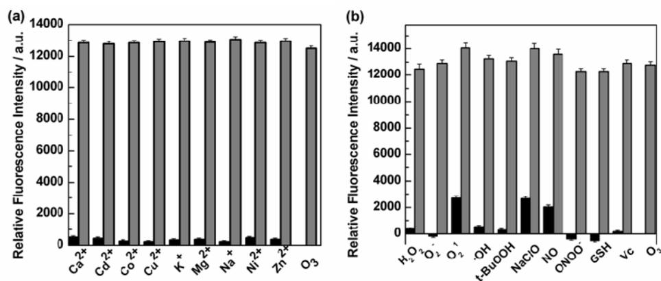
**Figure S5 (a)** The relative fluorescence response of 10  $\mu\text{M}$  probe to some metal ion (6
