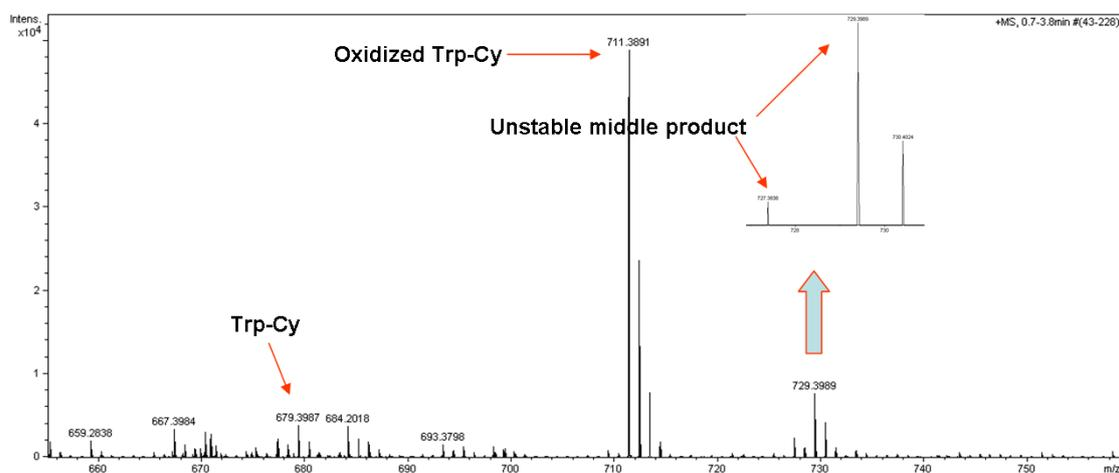
**Figure S6.** ESI-MS spectrum of the reaction solution of Trp-Cy and ozone
