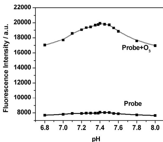
**Figure S2.** The relationship between the fluorescence intensity and pH value (10  $\mu$ M for Trp-Cy, 6  $\mu$ M for ozone and 30 mM for PBS)
