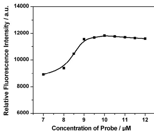
**Figure S4.** The relationship between of relative fluorescence intensity and the concentrations of the probe (6  $\mu\text{M}$  for ozone and 30 mM PBS, pH=7.4)
