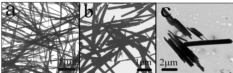
Fig. S1 TEM images of \text{CoC}_2\text{O}_4 NRs generated at different concentration of oxalic acid solution: (a) 0.01M, (b) 0.1 M, and (c) 0.5 M.
