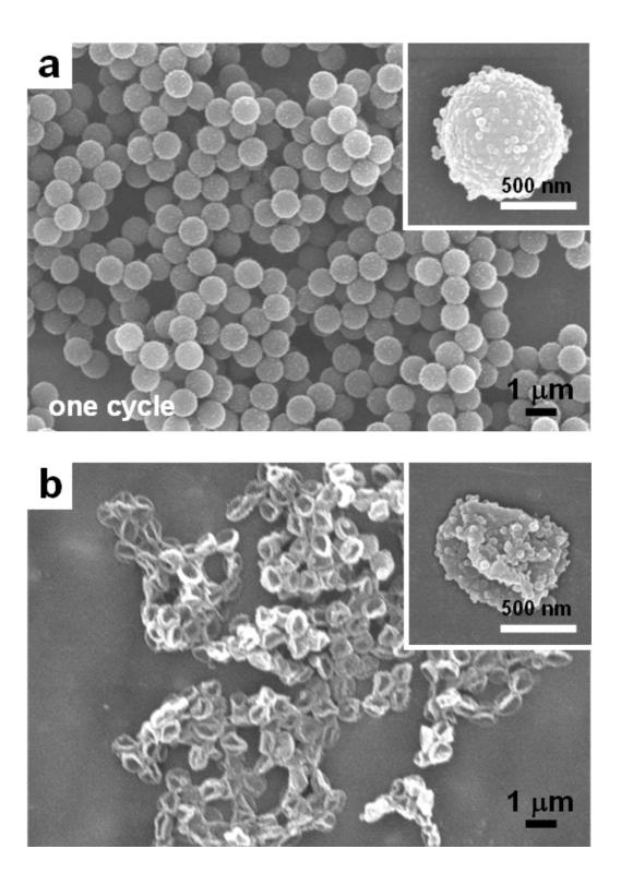
**Fig. S4** Broad range SEM images of (a) polystyrene@ZIF-8 core-shell microspheres with an average diameter of  $0.90 \pm 0.02 \ \mu m$  (s.d., n = 100) obtained by conducting only one ZIF-8 growth cycle and (b) hollow ZIF-8 particles obtained by etching the polystyrene cores of the polystyrene@ZIF-8 core-shell microspheres shown in (a). The insets are high-magnification images.
