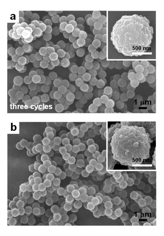
**Fig. S6** Broad range SEM images of (a) polystyrene@ZIF-8 core-shell microspheres with an average diameter of  $1.06 \pm 0.02 \ \mu m$  (s.d., n = 100) obtained by conducting three cycles of the ZIF-8 growth process and (b) hollow ZIF-8 particles obtained by etching the polystyrene cores of the polystyrene@ZIF-8 core-shell microspheres shown in (a). The insets are high-magnification images.
