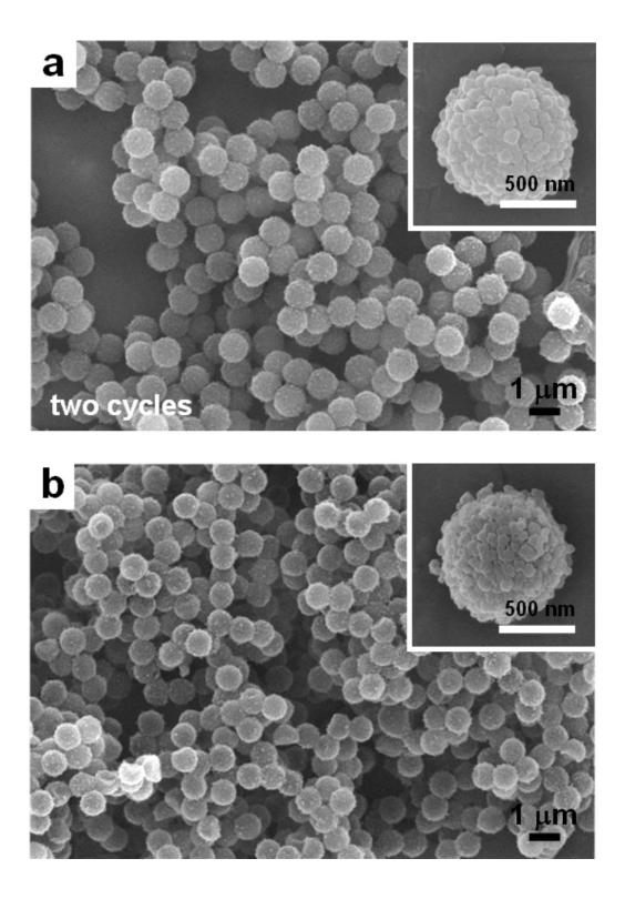
**Fig. S5** Broad range SEM images of (a) polystyrene@ZIF-8 core-shell microspheres with an average diameter of  $0.97 \pm 0.02 \ \mu m$  (s.d., n = 100) obtained by conducting two cycles of the ZIF-8 growth process and (b) hollow ZIF-8 particles obtained by etching the polystyrene cores of the polystyrene@ZIF-8 core-shell microspheres shown in (a). The insets are high-magnification images.
