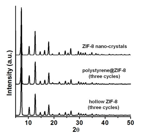
**Fig. S10** PXRD patterns for the hollow ZIF-8 microspheres (bottom), polystyrene@ZIF-8 coreshell microspheres (middle), and ZIF-8 nano-crystals (top). Polystyrene@ZIF-8 core-shell and hollow ZIF-8 microspheres were obtained by conducting three cycles of the ZIF-8 growth process. All three PXRD patterns are nearly identical.
