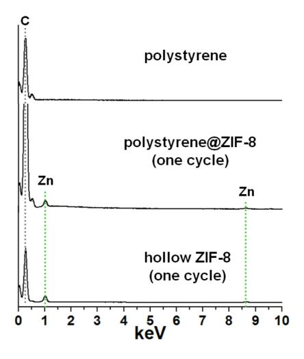
**Fig. S7** A series of EDX spectra of initial carboxylate-terminated polystyrene, polystyrene@ZIF-8 core-shell, and hollow ZIF-8 microspheres (top to bottom). Polystyrene@ZIF-8 core-shell and hollow ZIF-8 microspheres were obtained by conducting one cycle of the ZIF-8 growth process.
