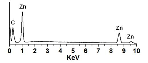
Fig. S3 EDX spectrum of ZIF-8 nano-crystals.
