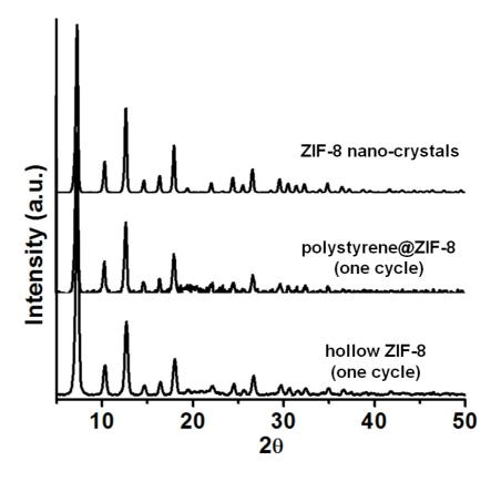
**Fig. S8** PXRD patterns for the hollow ZIF-8 microspheres (bottom), polystyrene@ZIF-8 core-shell microspheres (middle), and ZIF-8 nano-crystals (top). Polystyrene@ZIF-8 core-shell and hollow ZIF-8 microspheres were obtained by conducting one cycle of the ZIF-8 growth process. All three PXRD patterns are nearly identical.
