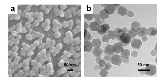
Fig. S2 (a) SEM and (b) TEM images of ZIF-8 nano-crystals.
