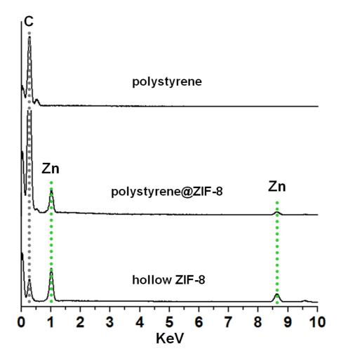
**Fig. S1** A series of EDX spectra of initial carboxylate-terminated polystyrene, polystyrene@ZIF-8 core-shell, and hollow ZIF-8 microspheres (top to bottom). Polystyrene@ZIF-8 core-shell and hollow ZIF-8 microspheres were obtained by conducting two cycles of the ZIF-8 growth process.
