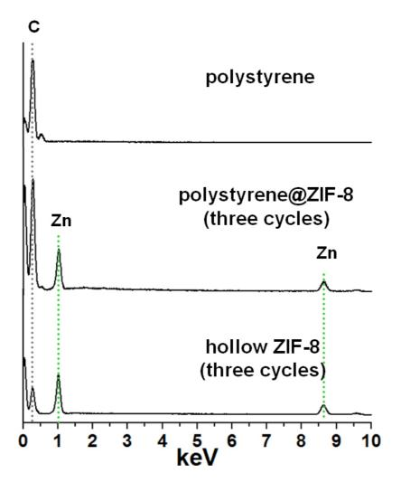
**Fig. S9** A series of EDX spectra of initial carboxylate-terminated polystyrene, polystyrene@ZIF-8 core-shell, and hollow ZIF-8 microspheres (top to bottom). Polystyrene@ZIF-8 core-shell and hollow ZIF-8 microspheres were obtained by conducting three cycles of the ZIF-8 growth process.
