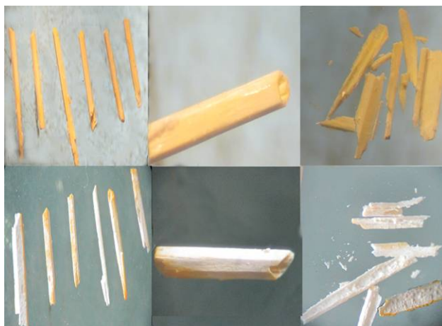
Fig. S1. Microscope images for (top) chemically synthesized \text{SiW}_{12}\text{-F} and (bottom) physically dyed \text{SiW}_{12}/\text{F} microtubes.
