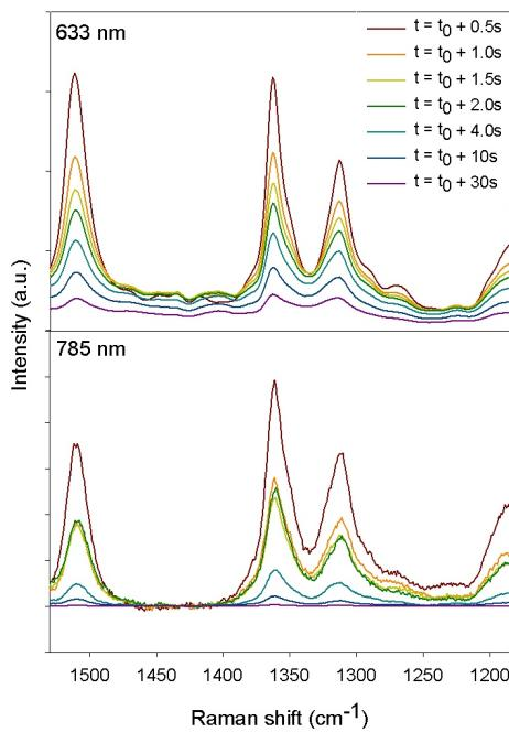
**Figure S5:** Comparison of the photo-degradation of Rh6G in air using a 785 nm laser (laser power 1 mW at sample) and a 633 nm laser (laser power 160 mW at sample) for  $\text{Al}_2\text{O}_3$ -supported Ag nanocubes.
