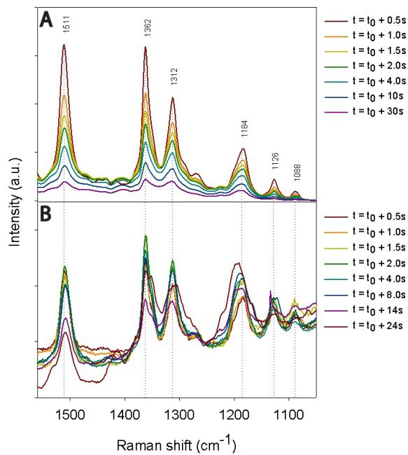
**Figure S4:** Comparison of the photo-degradation of Rh6G in air and in  $\text{N}_2$  using a 785 nm laser (laser power 1 mW at sample) for  $\text{Al}_2\text{O}_3$ -supported Ag nanocubes.
