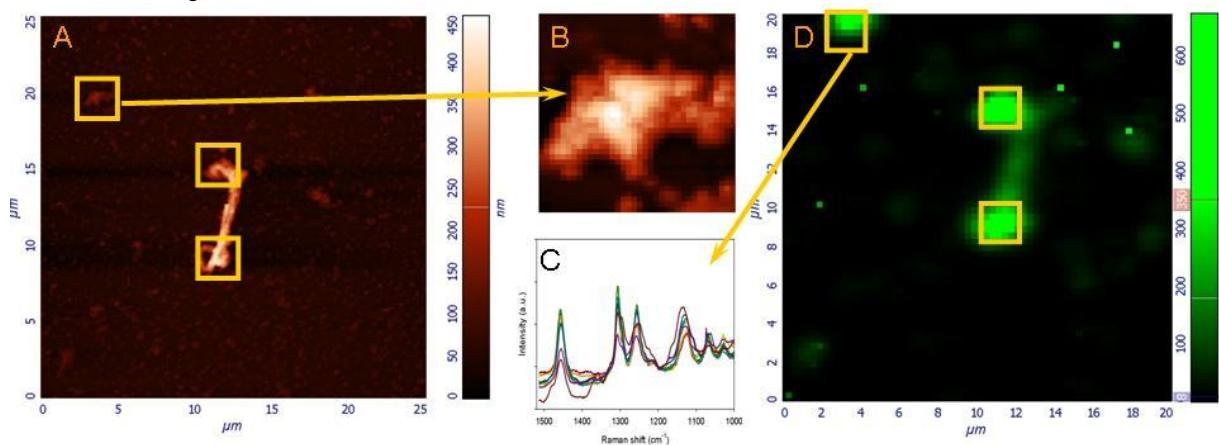
**Figure S3:** Simultaneous AFM and Raman imaging of an Al<sub>2</sub>O<sub>3</sub> wafer coated with Ag nano-cubes and Rh6G in N<sub>2</sub> using a 785 nm laser, laser power 160 mW at sample; (A) AFM height image of surface; (B) AFM magnification of an area over which Raman intensity was followed (scale bar = 400 nm); (C) Raman spectra followed over time from area B; (D) Raman intensity map of the Rh6G band at 1512 cm<sup>-1</sup>.
