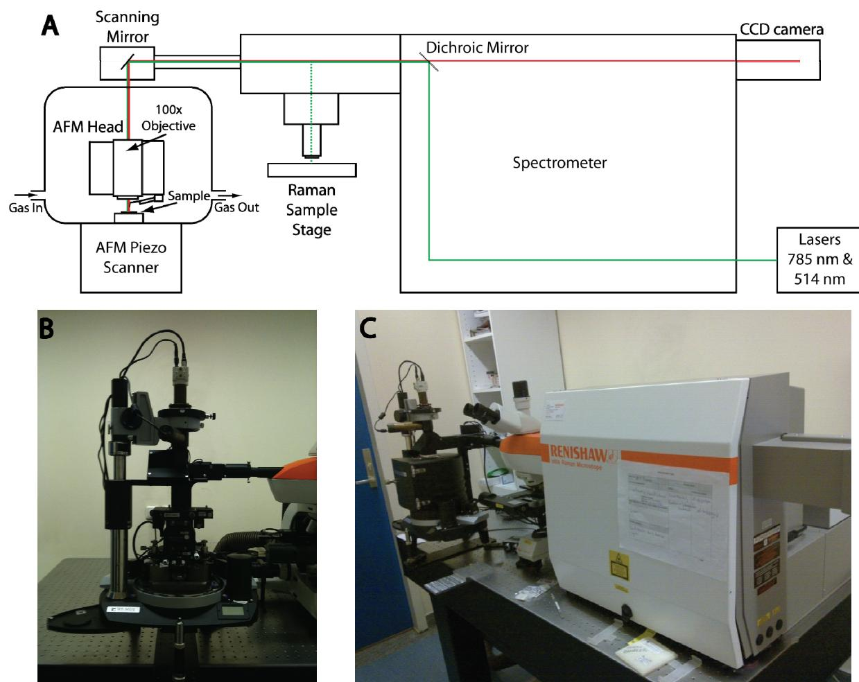
**Figure S1:** A) Set-up schematic and light path from lasers, through Renishaw InVia to NT-MDT NTEGRA Spectra and back to Renishaw RenCam CCD camera; B) photograph of the NTEGRA AFM head and laser coupling, and C) photograph of the integrated AFM-Raman setup with the in-situ chamber around the AFM head.
