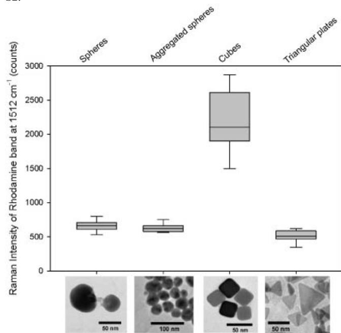
**Figure S2:** SERS enhancement of Rh6G for different Ag nano-particle morphologies. Measurements were carried out with a Renishaw InVia microscope using a 785 nm laser, 1 s exposure time, and a Leica 100x 0.85 NA objective.
