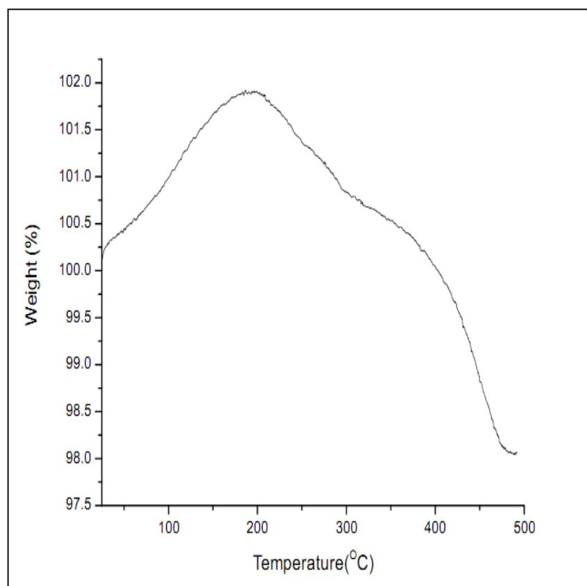
**Figure SI\_4** The TGA of CdS nanowire after pyridine exchange is shown in the figure. A weight gain of ~2 % is observed until 200°C. Further, beyond 200°C the material starts to lose weight as temperature is ramped up to 500°C.
