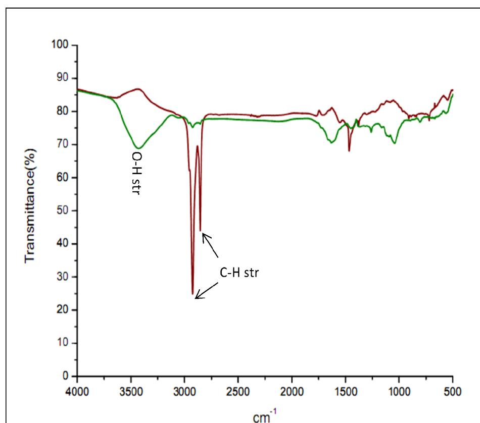
**Figure SI\_5** FTIR spectra of CdS nanowire before (red) and after (green) pyridine exchange is shown in the figure. The almost complete elimination of the C-H stretching frequency (noted between 3000-2800 cm<sup>-1</sup>) indicate the success of the ligand exchange.
