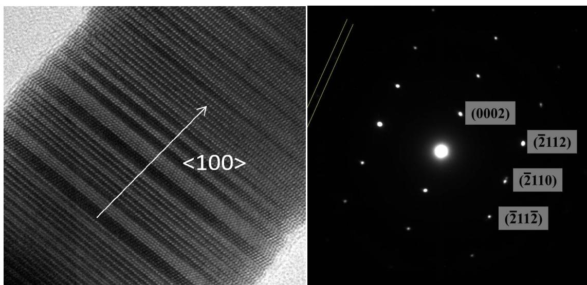
**Figure SI\_2** Figure SI\_2 (left) shows the HRTEM of a single crystalline CdS nanowire prepared using the SLS method. The growth direction of the nanowires matches with  $<100>$  of wurtzite CdS. Figure SI\_2 (right) shows the SAED pattern from the same nanowire. Points are indexed and matches with hexagonal CdS.
