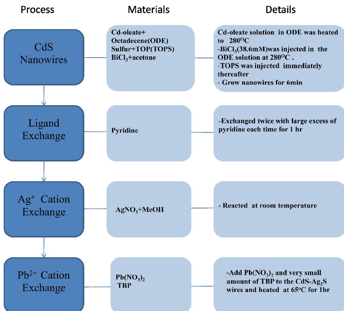
**Figure SI\_1** A process flow sheet for the synthesis of the 1D CdS/PbS nanowires.
