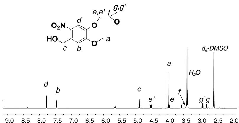
**Figure S2.**  $^1\text{H NMR}$  spectrum of (5-methoxy-2-nitro-4-(oxiran-2-ylmethoxy)phenyl)methanol (**1**) in  $d_6\text{-DMSO}$  (ppm).
