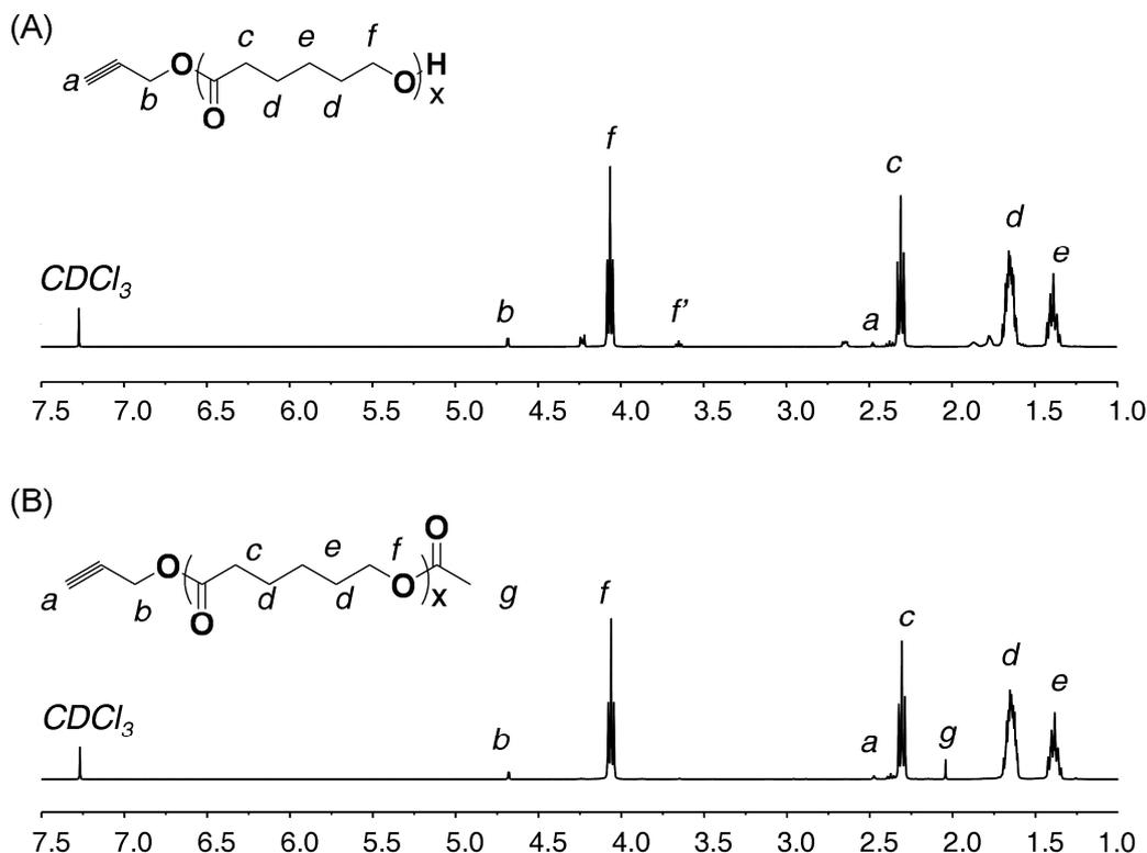
**Figure S4.** <sup>1</sup>H NMR spectra of (A) α-propargyl-ω-hydroxyl-poly(ε-caprolactone) and (B) α-propargyl-ω-acetyl-poly(ε-caprolactone) (**4**) in CDCl<sub>3</sub> (ppm).
