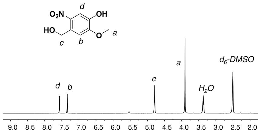
**Figure S1.**  $^1\text{H NMR}$  spectrum of 4-(hydroxymethyl)-2-methoxy-5-nitrophenol in  $\text{DMSO-}d_6$  (ppm).
