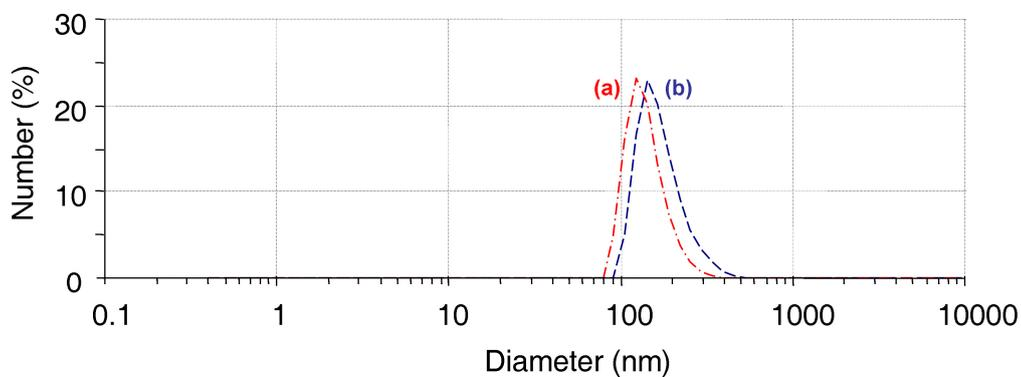
**Figure S9.** DLS analysis of the UV irradiated ECE micelle solution after stirring at 65 °C for 123 h (a) then cooling to room temperature for 24 h (b).
