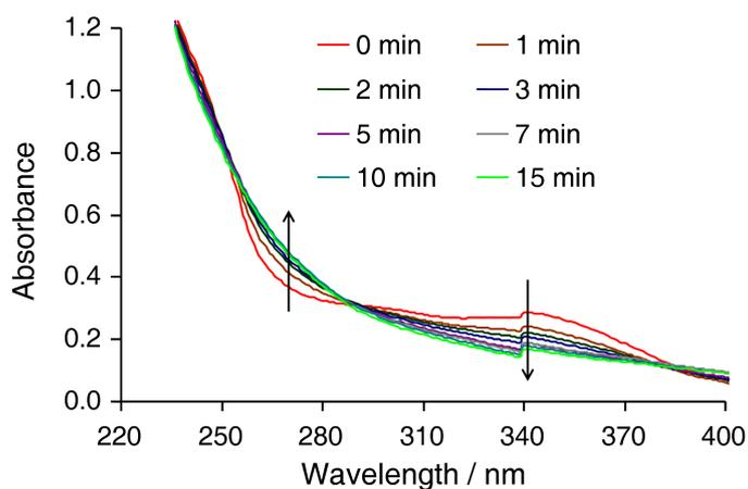
**Figure S7.** UV-vis absorption spectra of the ECE polymer assemblies after UV irradiation for different time periods.
