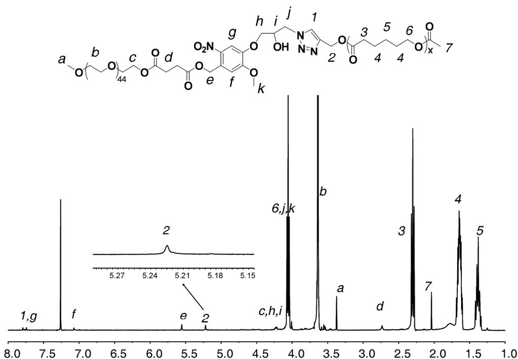
**Figure S5.**  $^1\text{H}$  NMR spectrum of mPEG<sub>45</sub>-NB-PCL (**5**) in CDCl<sub>3</sub> (ppm).
