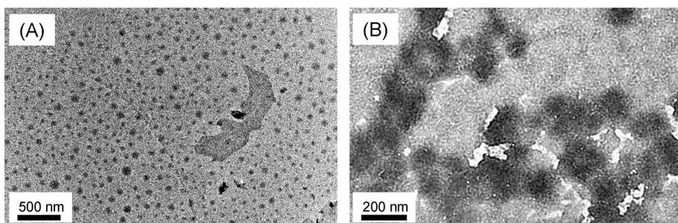
**Figure S8.** TEM images of (A) the ECE micelles without UV irradiation but stirred at 65 °C for 123 h and (B) assemblies after UV irradiation for 15 min and stirred at 65 °C for 24 h.
