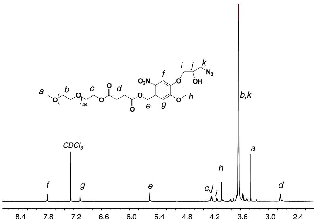
**Figure S3.** <sup>1</sup>H NMR spectrum of 4-(3-azido-2-hydroxypropoxy)-5-methoxy-2-nitrobenzyl mPEG<sub>45</sub>-succinate (**3**) in CDCl<sub>3</sub> (ppm).
