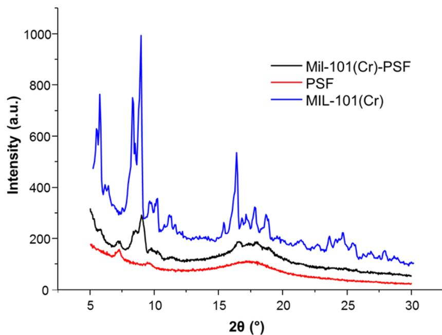
**Fig. S4** X-ray powder diffraction pattern; (black: 16% MIL-101-PSF membrane of 59  $\mu\text{m}$  thickness).
