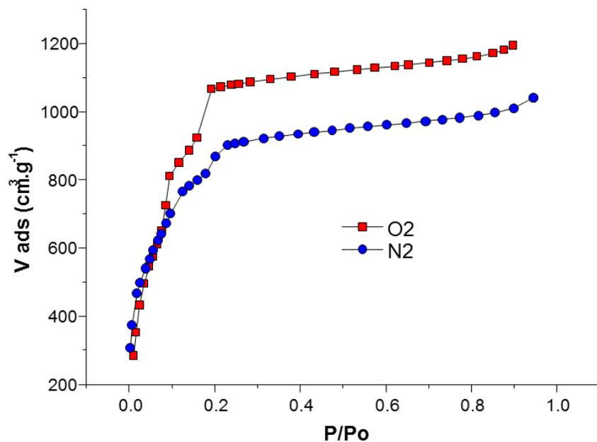
**Fig. S5** O<sub>2</sub> and N<sub>2</sub> adsorption isotherms of a synthesized and activated MIL-101 sample; These sorption isotherms were fitted by the Brunauer–Emmett–Teller (BET) and Langmuir (L) equations (at  $p/p_0 = 0.06 - 0.16$ ) to give  $S_{\text{BET}}$  (3239 m<sup>2</sup>/g) and  $S_{\text{L}}$  (4617 m<sup>2</sup>/g) surface areas and a total pore volume of 1.61 cm<sup>3</sup>/g.
