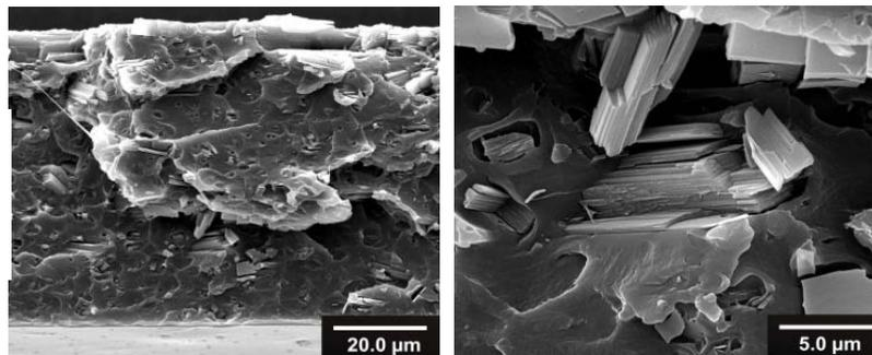
**Fig. S2** SEM cross-sections of MOF-PSF membranes based on 400 mg of PSF with 8 wt% loadings of selected MOFs (as indicated).
