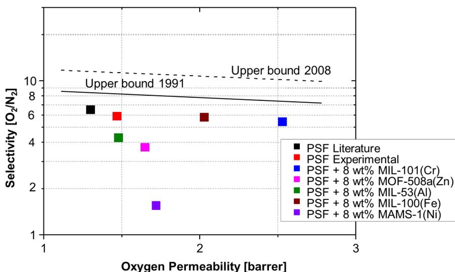
**Fig. S1** O<sub>2</sub>/N<sub>2</sub> Separation performance of selected MOFs-PSF mixed-matrix membranes. The Robeson upper bounds for polymer performance as defined in 1991<sup>3</sup> and 2008<sup>4</sup> are shown.
