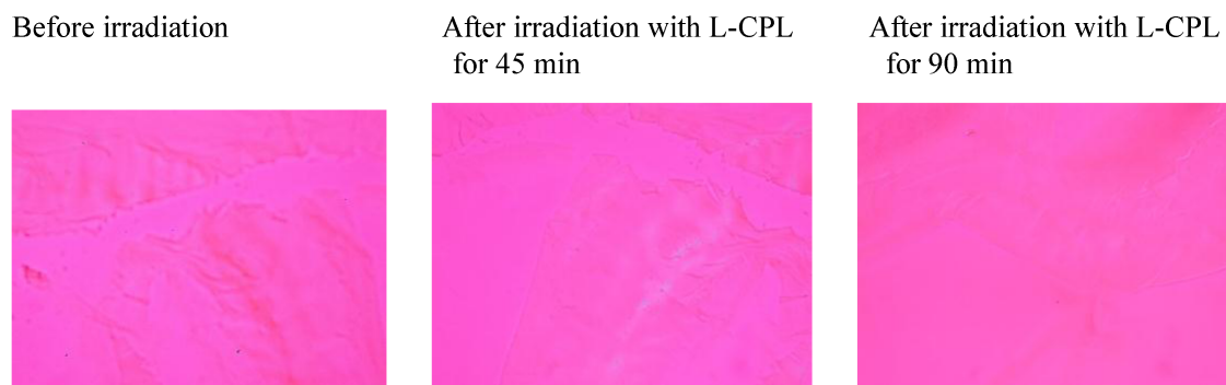
Fig. S8. Polarized optical micrographs of PDOF before and after irradiation with L-CPL from a 500-W Hg-Xe lamp for 45 min and for 90 min. Irradiation was conducted on a glass plate.
