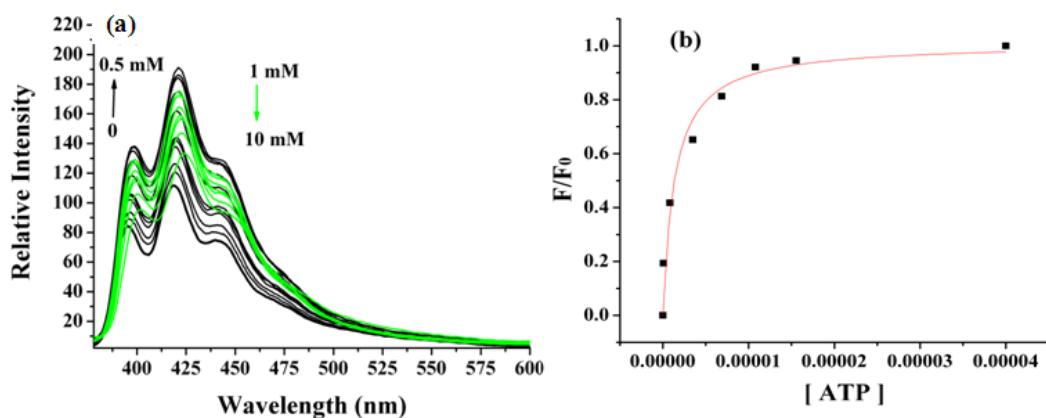
**Figure S5 .** Emission spectra (excitation at 367 nm) of receptor **1** (10  $\mu$ M) upon addition of Na salt of ATP at pH 7.4 (10 mM phosphate buffer) and the corresponding binding isotherm.
