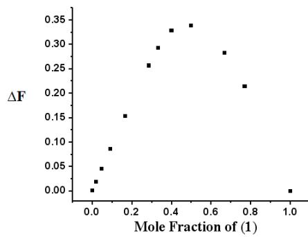
**Figure S7.** Assessment of the stoichiometry of the ATP complex of **1** via Job plot analysis;  $[1] + [\text{ATP}] = 10 \mu\text{M}$ , pH 7.4 (10 mM phosphate buffer), 25°C.
