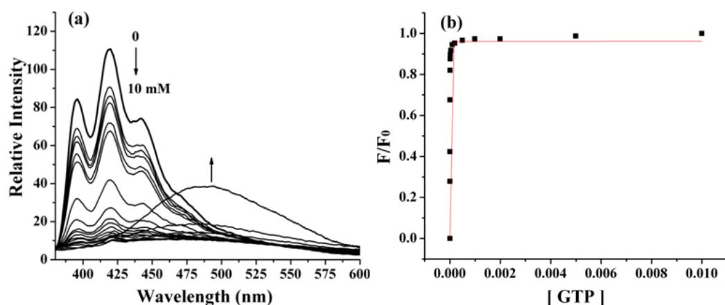
**Figure S4.** Emission spectra (excitation at 367 nm) of receptor **1** (10  $\mu$ M) upon addition of Na salt of GTP at pH 7.4 (10 mM phosphate buffer) and the corresponding binding isotherm.
