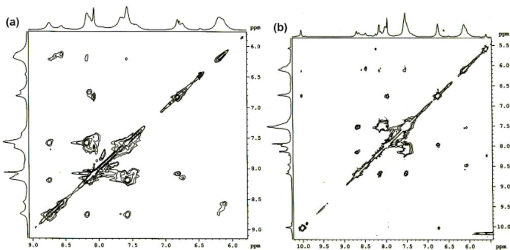
**Figure S8.** 500 MHz NOESY spectrum of **1** with 1 eq. of (a) GTP (b) ATP in DMSO-d<sub>6</sub>.
