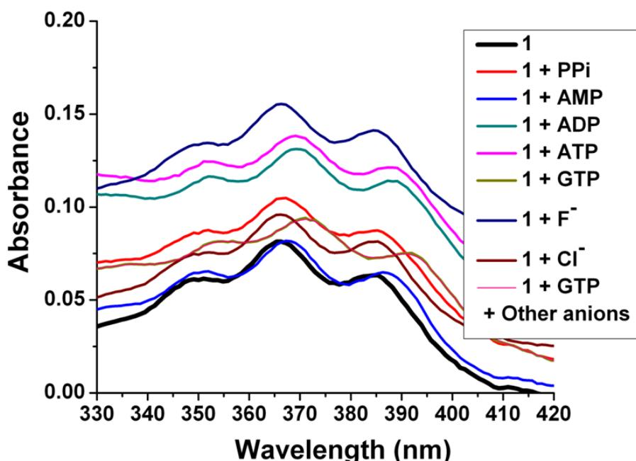
**Figure S3.** Absorption spectra of **1** (10  $\mu$ M) upon the addition of sodium salts of pyrophosphate (PPi), AMP, ADP, ATP, GTP and TBA salts of F<sup>-</sup> and Cl<sup>-</sup> (100 equiv) at pH 7.4 (10 mM phosphate buffer).
