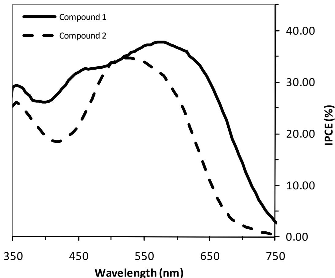
**Figure S6** The Incident Photon Collection Efficiency (IPCE) data were collected using an Oriel 150W Xe lamp coupled to a monochromator and an optical fibre. The output of the optical fibre was focussed to give a beam that was contained within the area of the device. The IPCE was calibrated with a standard, unfiltered Si cell and the data was corrected to the output of the calibrated AM1.5 solar simulator response. IPCE data are for the **bold** devices described in Section 7.2 and 7.3.
