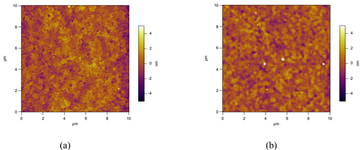
**Figure S8** AFM images of PC<sub>61</sub>BM-blended films of compound **2** spun from different solvents. Unit for the AFM images is  $\mu\text{m}$ . Solvents were chlorobenzene (a) and chloroform (b). Solution concentrations, blend ratios and device power conversion efficiencies were as indicated below.
