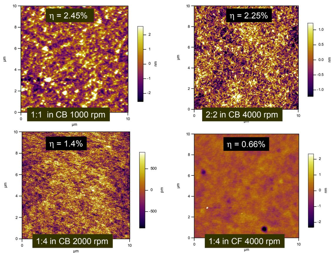
**Figure S7** AFM images of PC<sub>61</sub>BM-blended films of compound 1 spun at various spin speeds in different solvents. Unit for the AFM images is μm. CB=chlorobenzene, CF=chloroform, blend ratios and device power conversion efficiencies are as indicated.
