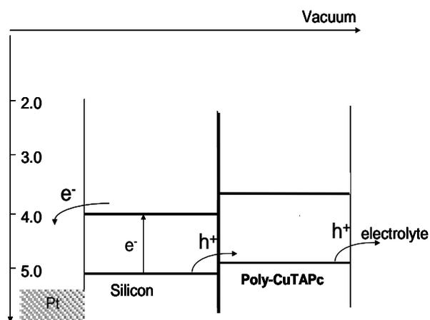
Figure S7 Energy band diagram of a SiNWs/poly-CuTAPc heterojunction.
