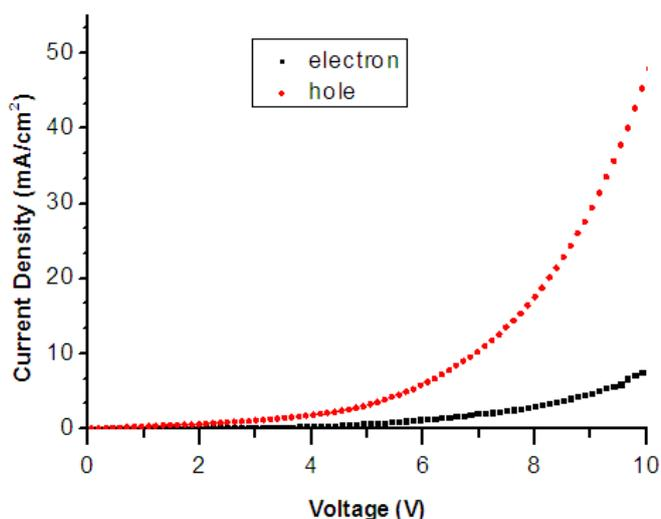
Figure S3 Current density versus voltage for the hole-only and electron-only devices of
