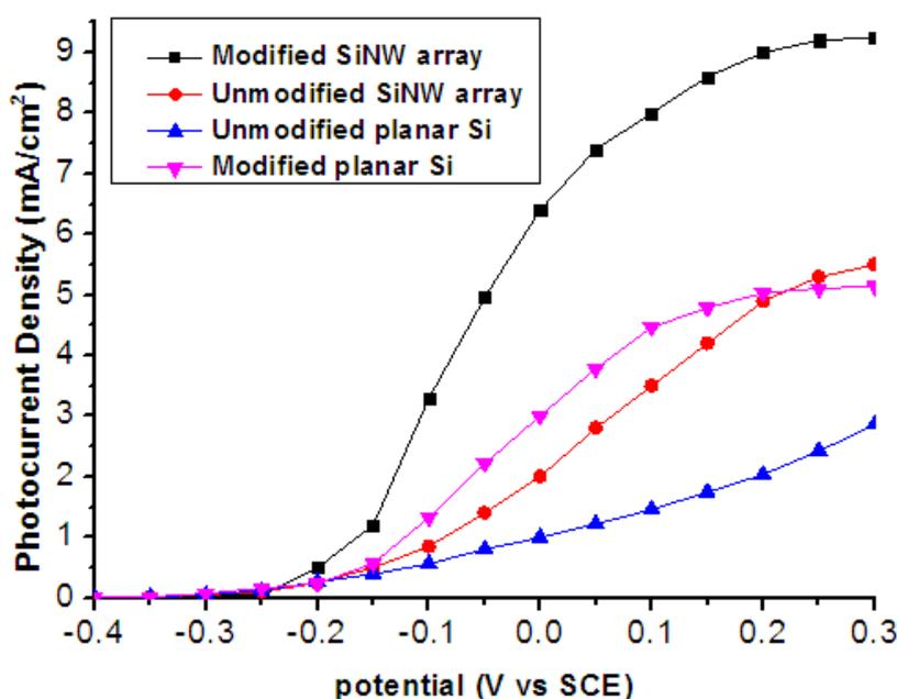
Figure S6 Photocurrent densities for modified and unmodified planar silicon and SiNW array with the same condition as figure 2.
