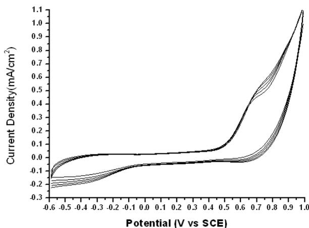
Figure S2 Repeated cyclic voltammograms recorded during the first 5 cycles of electropolymerization, scan rate, 100 mV/s; initial potential, +1.000 V; working electrode, OH-terminated n-type SiNWs arrays.
