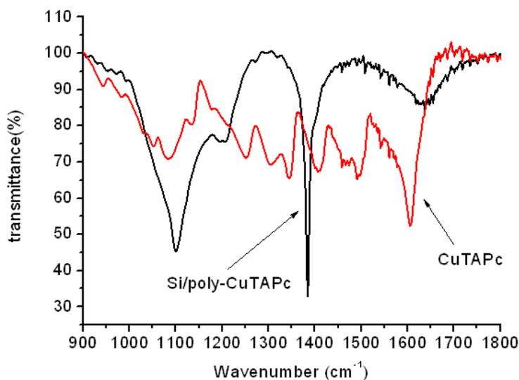
Figure S4 The IR of Si/poly-CuTAPc coaxial core-shell nanowires and CuTAPc.
