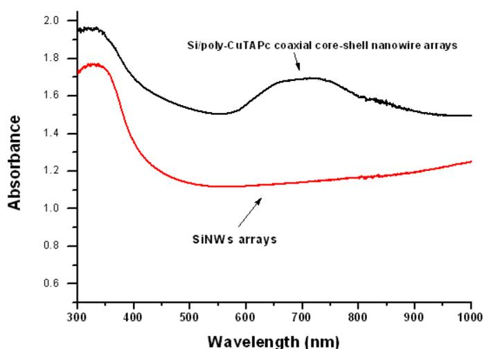
Figure S5 The UV-visible absorption of Si/poly-CuTAPc coaxial core-shell nanowire arrays and Si NWs arrays.
