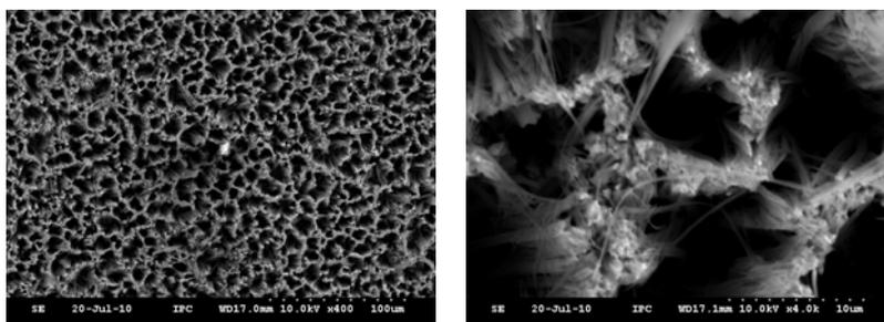
Figure S1 The SEM image of SiNWs arrays.
