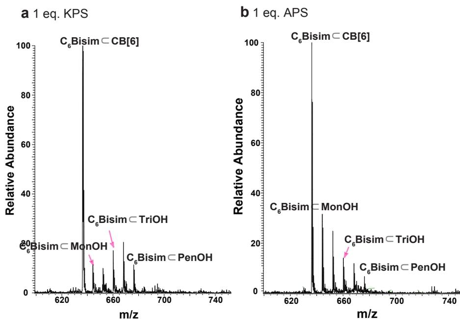
Figure 2: ESI-MS spectra depicting a) reaction mixture of CB[6] and 1 equivalent of KPS at time = 6 h; b) reaction mixture of CB[6] and 1 equivalent of APS at time = 12 h.
