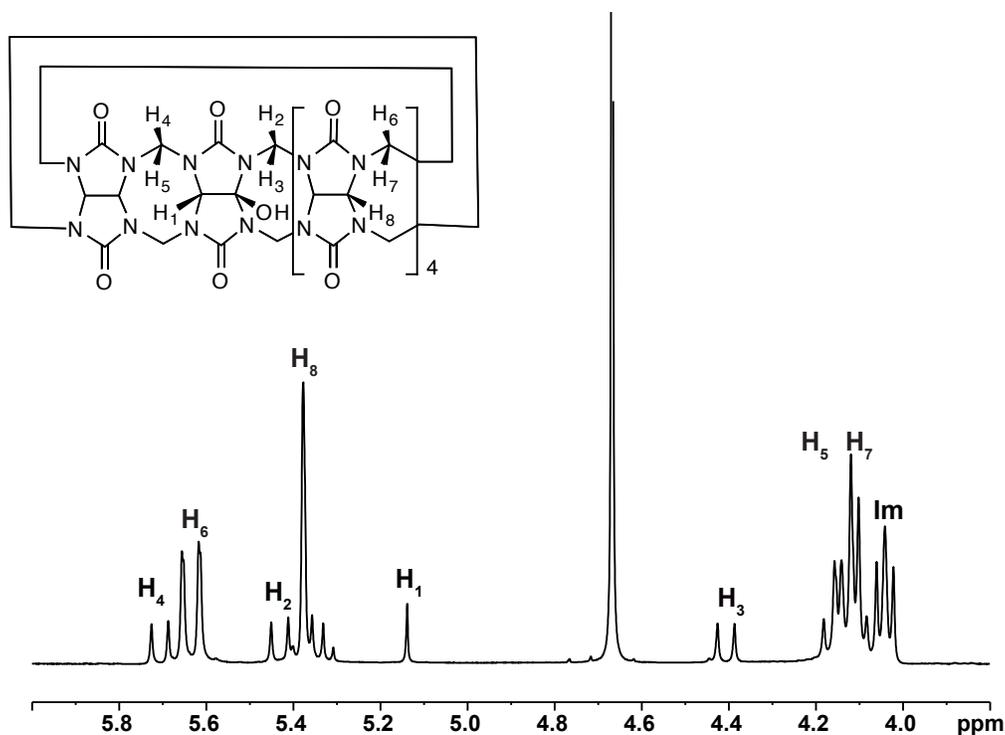
Figure 3: Partial <sup>1</sup>H NMR spectrum of 1C MonOH
