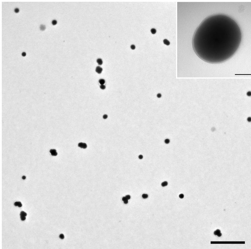
Figure S4. Transmission electron microscopy image of TCPP-containing silica NSs: scale bar 2  $\mu\text{m}$ . (Inset) Magnification: scale bar 100 nm.
