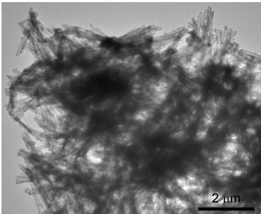
Figure S3. Transmission electron microscopy images of silica/TCPP HNTs.
