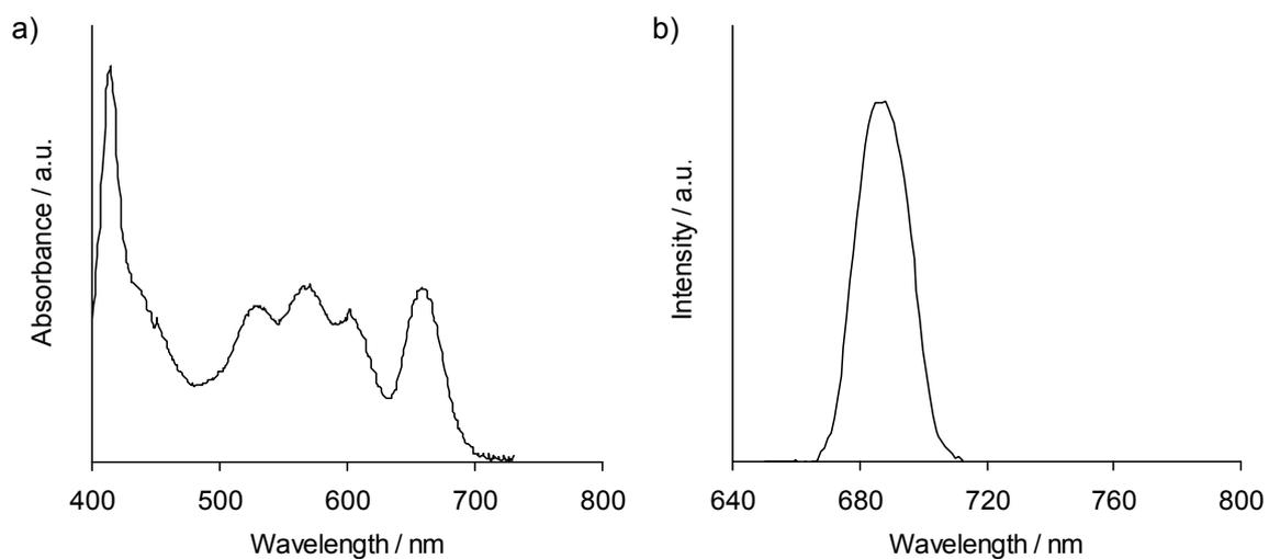
Figure S8. (a) Absorption spectrum of TCPP-containing silica NSs in PBS. (b) Fluorescence spectrum of TCPP-containing silica NSs in PBS:  $\lambda_{\text{ex}} = 658 \text{ nm}$ .
