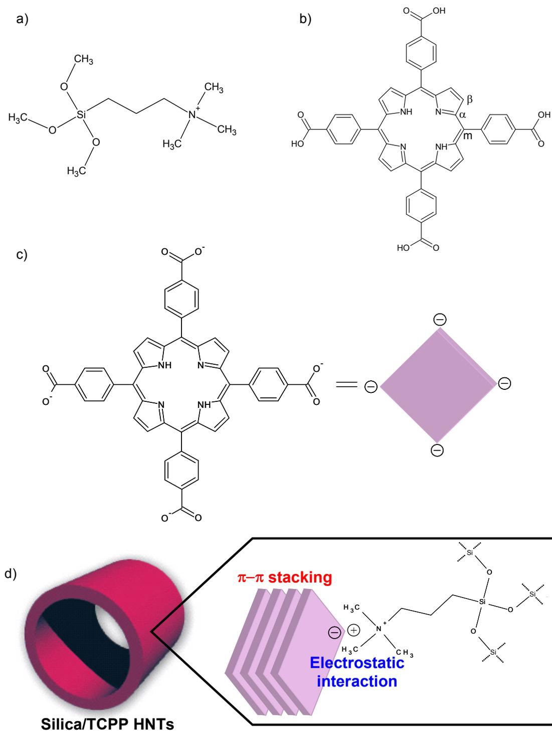
Figure S1. Chemical structures of (a) TMAPS, (b) TCPP and (c) the TCPP anion. (d) Schematic representation of silica/TCPP HNTs.
