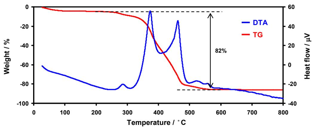
Figure S6. DTA and TG curve of silica/TCPP HNTs.
