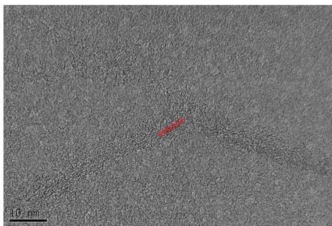
Figure S3. HRTEM image of the ripples on the sulfonated graphene (G-SO 3 H) sheets.
