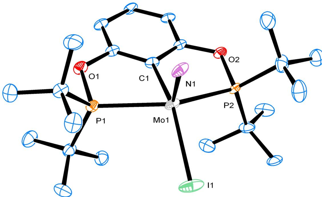
Figure S1. Thermal ellipsoid representation of (*t*-BuPOCOP)Mo(I)(N)(H) (**4**) at 50% probability level. H atoms and whole molecule disorder are omitted. Selected bond distances (Å) and angles (°): Mo1–C1 2.204(4), Mo1–P1 2.529(2), Mo1–P2 2.525(2), Mo1–I1 2.7537(6), Mo1–N1 1.643(3), C1–Mo1–I1 152.44(10), P1–Mo1–P2 145.30(9), I1–Mo1–N1 105.75(14).
