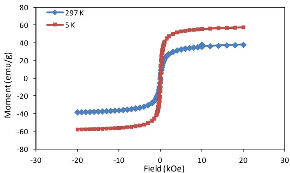
**Fig. S4.** Field-dependent magnetization of NP 2 at 297 K (blue line) and 5 K (red line) using SQUID. NP 2 exhibited superparamagnetic properties as evident from the absence of a hysteresis loop.
