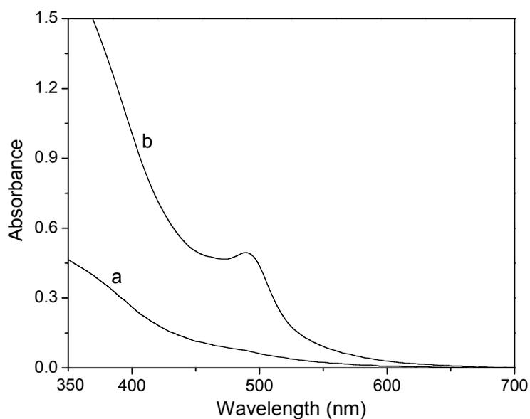
**Fig. S6.** UV-vis absorption curves of  $\beta$ -CD conjugated SPION (NP2, curve a) and FITC-labelled  $\beta$ -CD conjugated SPION (FITC-NP2, curve b). The nanoparticle concentration is 0.4 mg/mL in both cases. Based on the UV-vis absorbance, there are on average 16 FITC on each FITC-NP 2.
