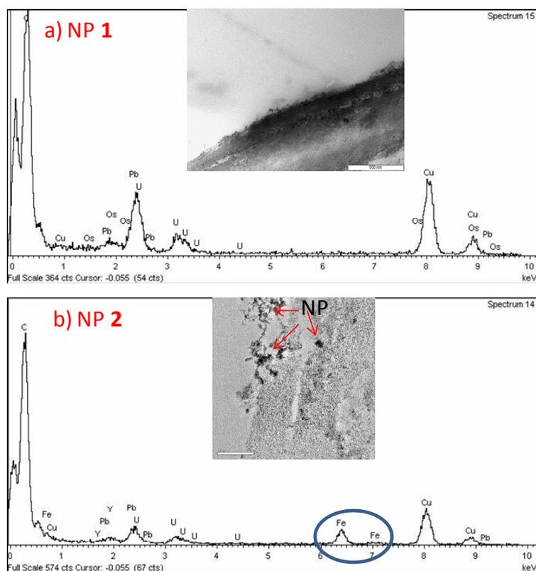
**Fig. S8.** X-ray photoelectron spectroscopy spectra of atherosclerotic tissues incubated with a) NP 1 and b) NP 2. Iron was clearly detected in the lower spectrum supporting the observation of NP in the corresponding TEM images. Cu was from the copper grid, U was from the uranium acetate staining, Os was from the osmium tetroxide used for tissue processing.
