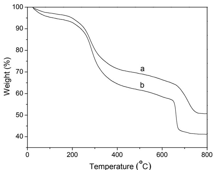
**Fig. S2.** TGA of iron oxide nanoparticles of NH<sub>2</sub>-NP 1 (curve a) and NP 2 (curve b). NP 2 showed an extra 10% weight loss when the sample was heated to 800 °C due to  $\beta$ -CD conjugation. Based on TGA data before and after  $\beta$ -CD conjugation, it can be determined that 42% of the NP 2 weight came from Fe<sub>3</sub>O<sub>4</sub> core, 39% came from the dextran coating and 19% was due to  $\beta$ -CD.
