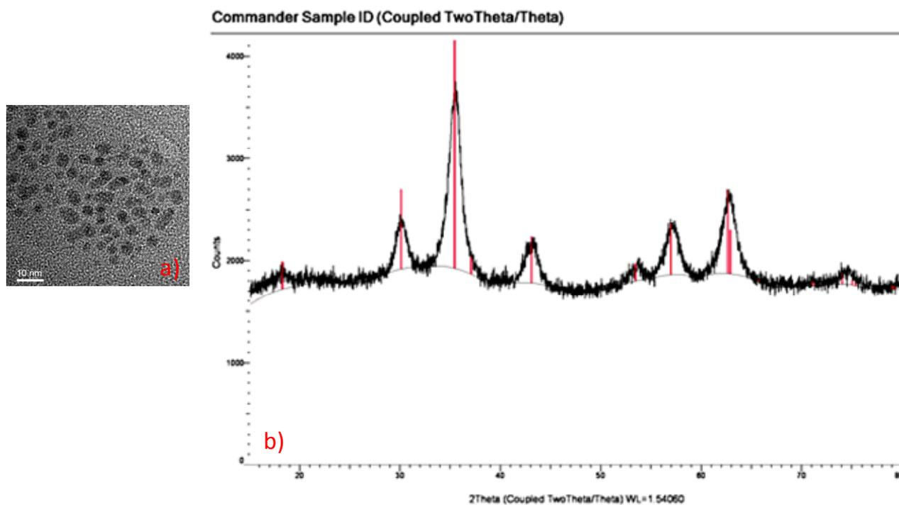
**Fig. S1.** a) TEM image of  $\beta$ -CD conjugated SPION (NP 2) showing average core size of the NP was 6 nm. b) Power XRD spectrum of NP 2 confirming the core of NP 2 was Fe<sub>3</sub>O<sub>4</sub> magnetite. The red lines are the magnetite peak patterns from the database.
