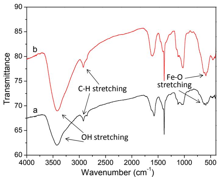
**Fig. S3.** FTIR of iron oxide nanoparticles before (curve a) and after (curve b)  $\beta$ -CD conjugation.
