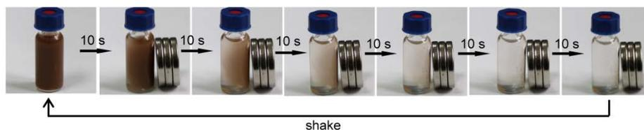
Figure S1. Dispersing and collection of the MSP microspheres in water with the help of a common magnet.
