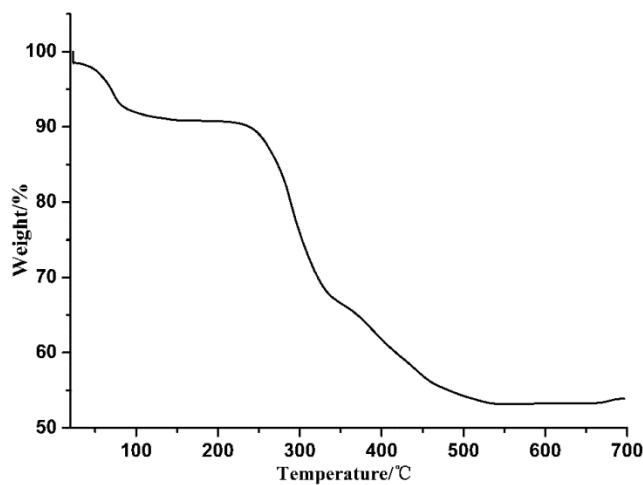
**Figure S6:** TGA of **1** in a N<sub>2</sub> flow.
