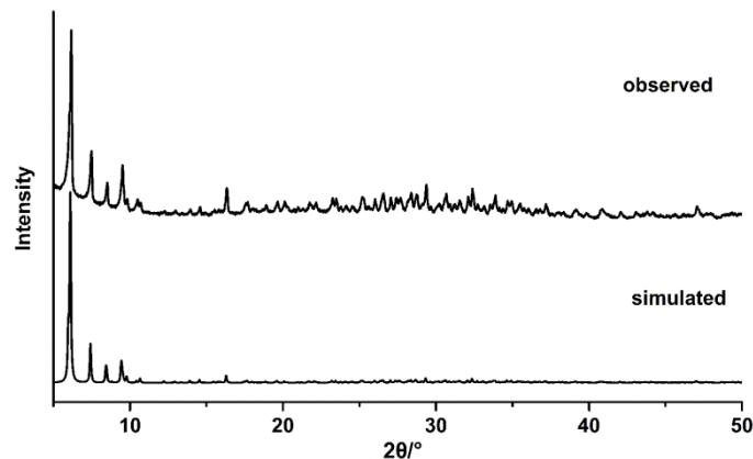
**Figure S7:** Simulated and observed powder X-ray diffraction (PXRD) of **1**.
