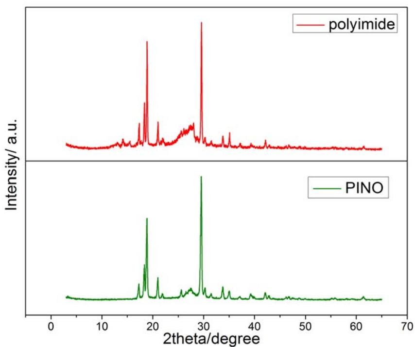
Fig. S4 XRD spectra of polyimide and PINO
