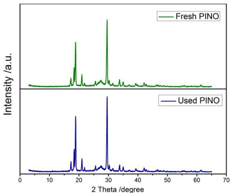
Fig. S6 XRD of fresh PINO and used PINO
