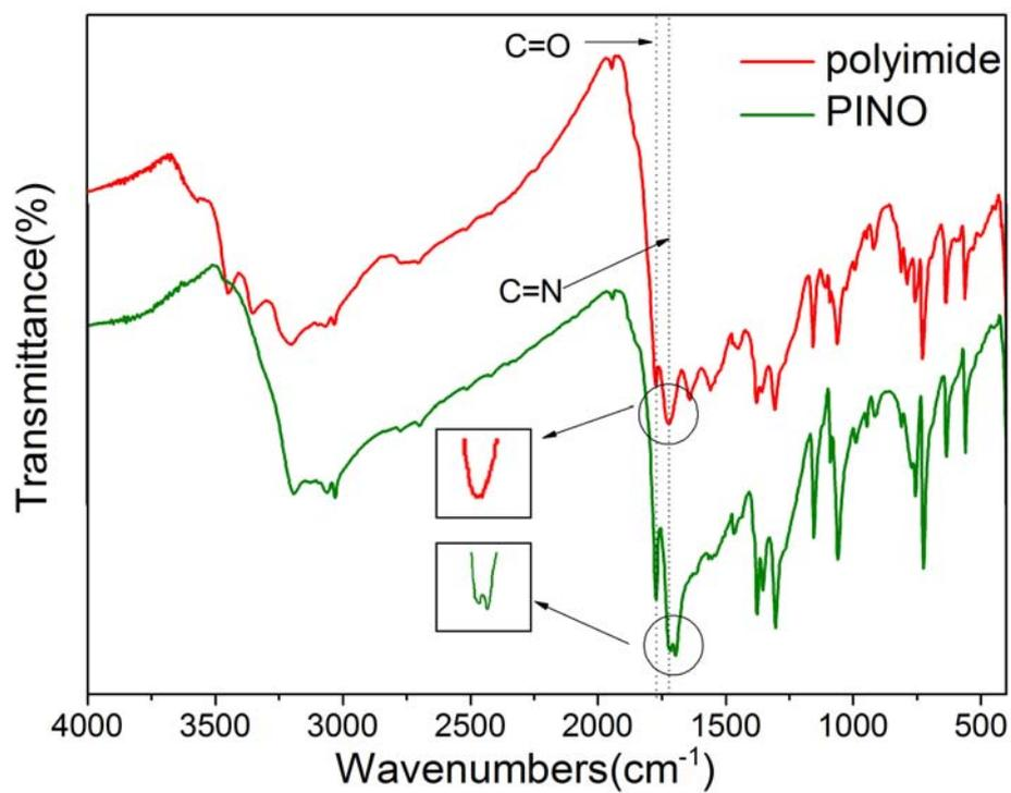
Fig. S3 FTIR spectra of polyimide and PINO
