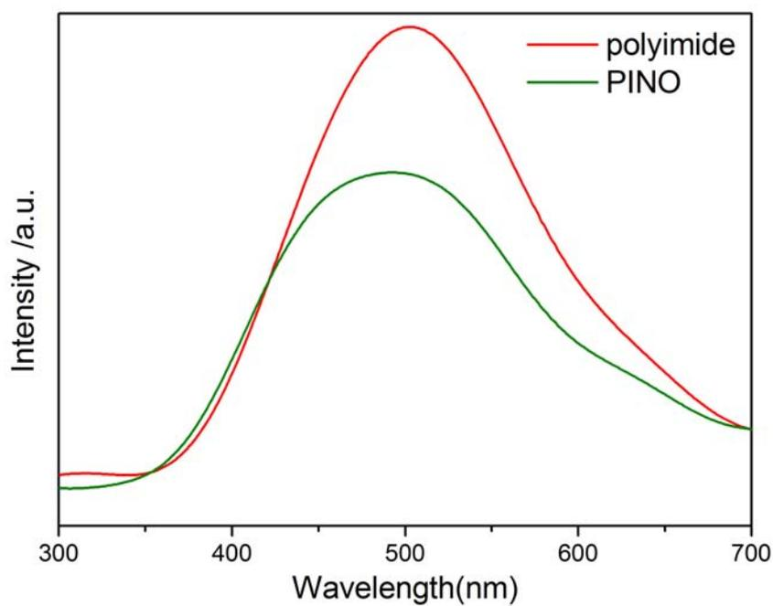
Fig. S8 Photoluminescence spectra of polyimide and PINO
