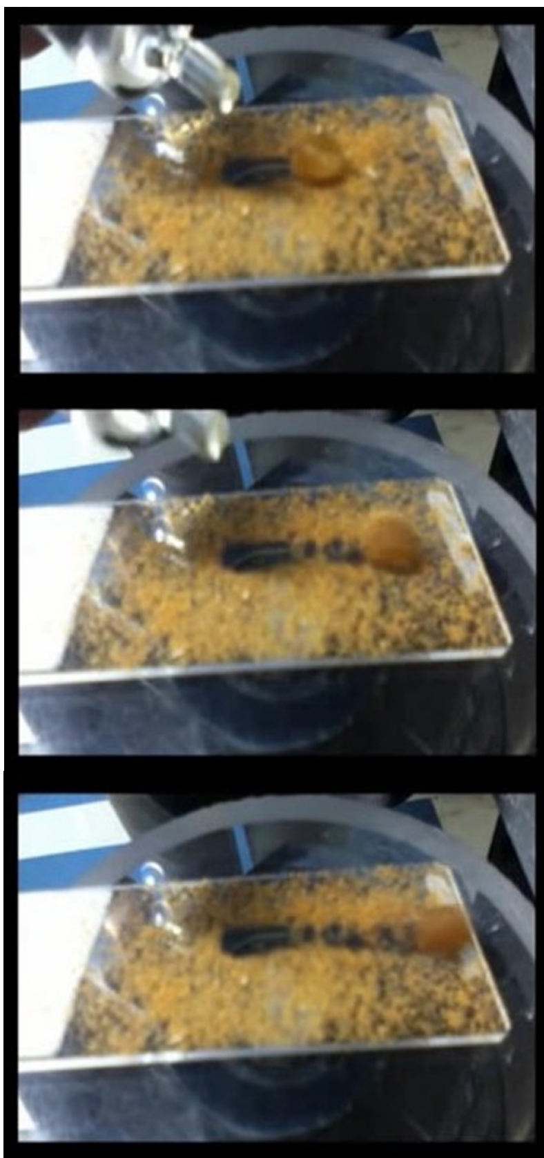
Figure ESI7. Sequence of self-cleaning properties of the obtained coatings.
