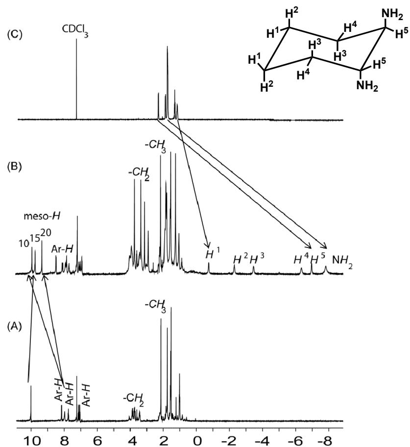
**Figure S3.** <sup>1</sup>H NMR spectra of (A) **1**, (B) **1**•CHDA and (C) (1*S*,2*S*)-CHDA at 295 K in CDCl<sub>3</sub>. Inset shows the proton numbering scheme of CHDA ligand.
