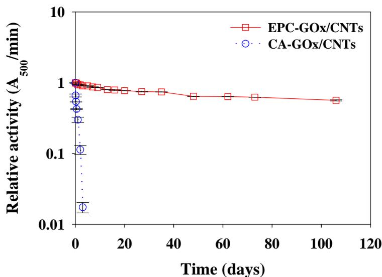
**Figure S4.** Stabilities of EPC-GOx/CNTs and covalently-attached GOx/CNTs (CA-GOx/CNTs) at 40°C. The relative activity represents the ratio of residual activity at each time point to the initial activity of each sample.
