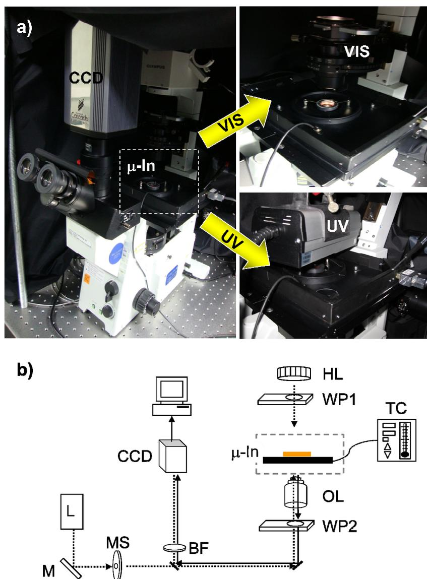
**Fig. S4** (a) A photograph of the integrated TIRFM and Nomarski DIC system. (b) Schematic diagram of the integrated system. Indicators: L, laser; M, mirror; MS, mechanical shutter; BF, bandpass filter; HL, halogen light lamp; WP, Wollaston prism; TC, temperature controller; OL, objective lens; CCD, charge-coupled device;  $\mu$ -In, microcell incubator.
