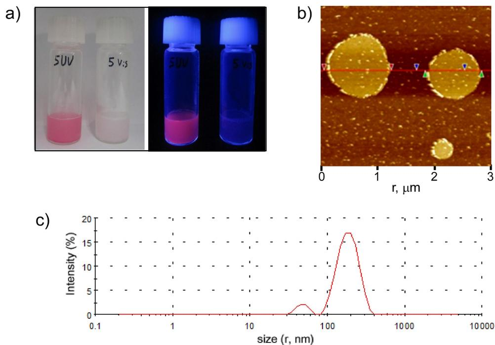
**Fig. S2** (a) Photographs of DC-Chol/DPPC solution containing compound **1**. Solutions in the left and right vials were UV- and visible-light irradiated, respectively. (b) Atomic force microscopy (AFM) analysis was performed to confirm liposome formation and the size distribution of liposomes. (c) Dynamic light scattering (DLS) analysis of compound **1** when integrated into a DC-Chol/DPPC liposome complex.
