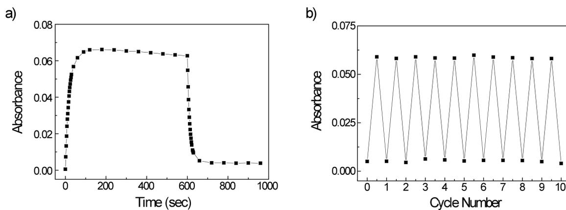
**Fig. S1.** (a) Time-course measurement of the absorption spectrum of compound **1** ( $1.0 \times 10^{-5}$  M in ethyl acetate at room temperature) upon UV irradiation (312 nm, 1-600 seconds), followed by visible light illumination (520 nm, 600-1000 sec). (b) UV absorption switching of **1** ( $1.0 \times 10^{-5}$  M in ethyl acetate at room temperature) between ring-open and ring-closed states upon alternative illumination with UV and visible light as monitored at 520 nm.
