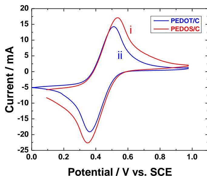
**Figure S6.** The electrochemical redox reaction on (i) PEDOS/C and (ii) PEDOT/C surface measured in 0.1  $\text{FeCl}_3$  and 0.1 HCl. The electrochemically accessible surface area (obtained from integration of the CV curve) of PEDOS/C electrode is 1.4 times larger than that of PEDOT/C electrode.
