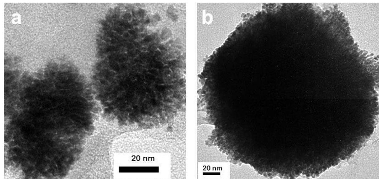
**Figure S4.** TEM images of Pt nanoparticles deposited on (a) PEDOS/C and (b) PEDOT/C electrodes.
