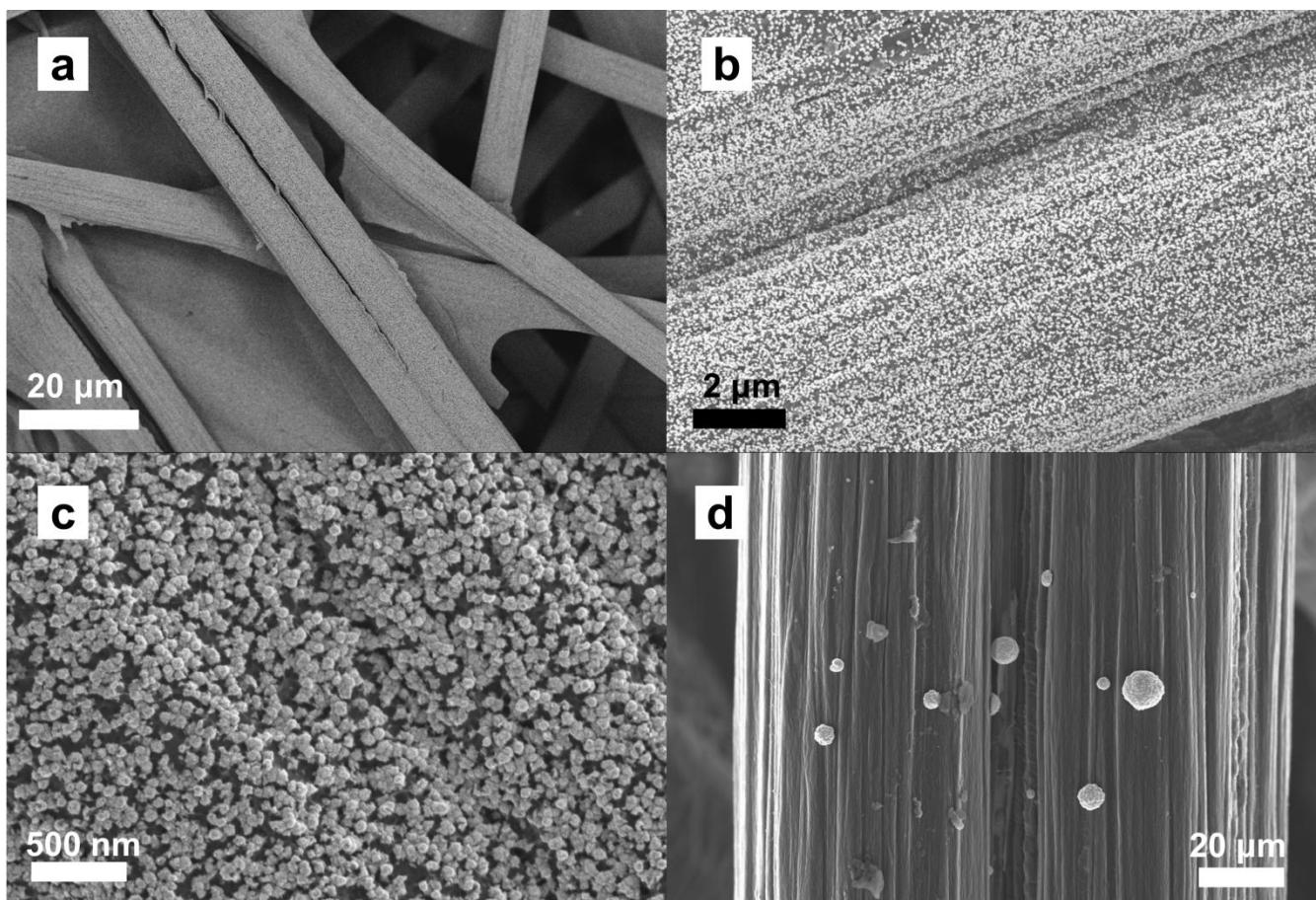
**Figure S2.** Additional SEM images of Pt nanoparticles on (a-c) PEDOS/C electrode and (d) on bare carbon paper electrode.
