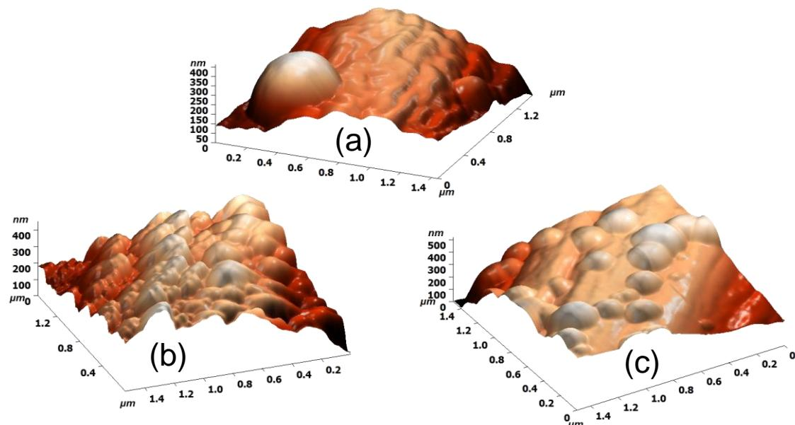
**Figure S3.** 3D surface AFM images of Pt nanoparticles on (a) bare carbon paper, (b) PEDOS/C and (c) PEDOS/C electrodes (only plane level correction was applied on the raw data).
