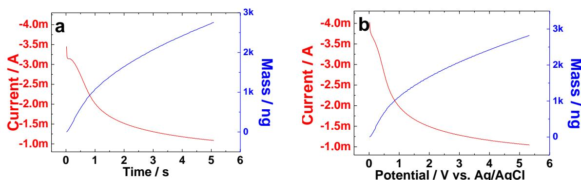
**Figure S5.** The EQCM study of Pt deposition on (a) PEDOS and (b) PEDOT coated gold crystal. At a deposition charge of 8.5 mC, the deposited mass of Pt on a PEDOS coated gold crystal is 2.76  $\mu\text{g}$ , whereas on a PEDOT surface it is 2.82  $\mu\text{g}$ .
