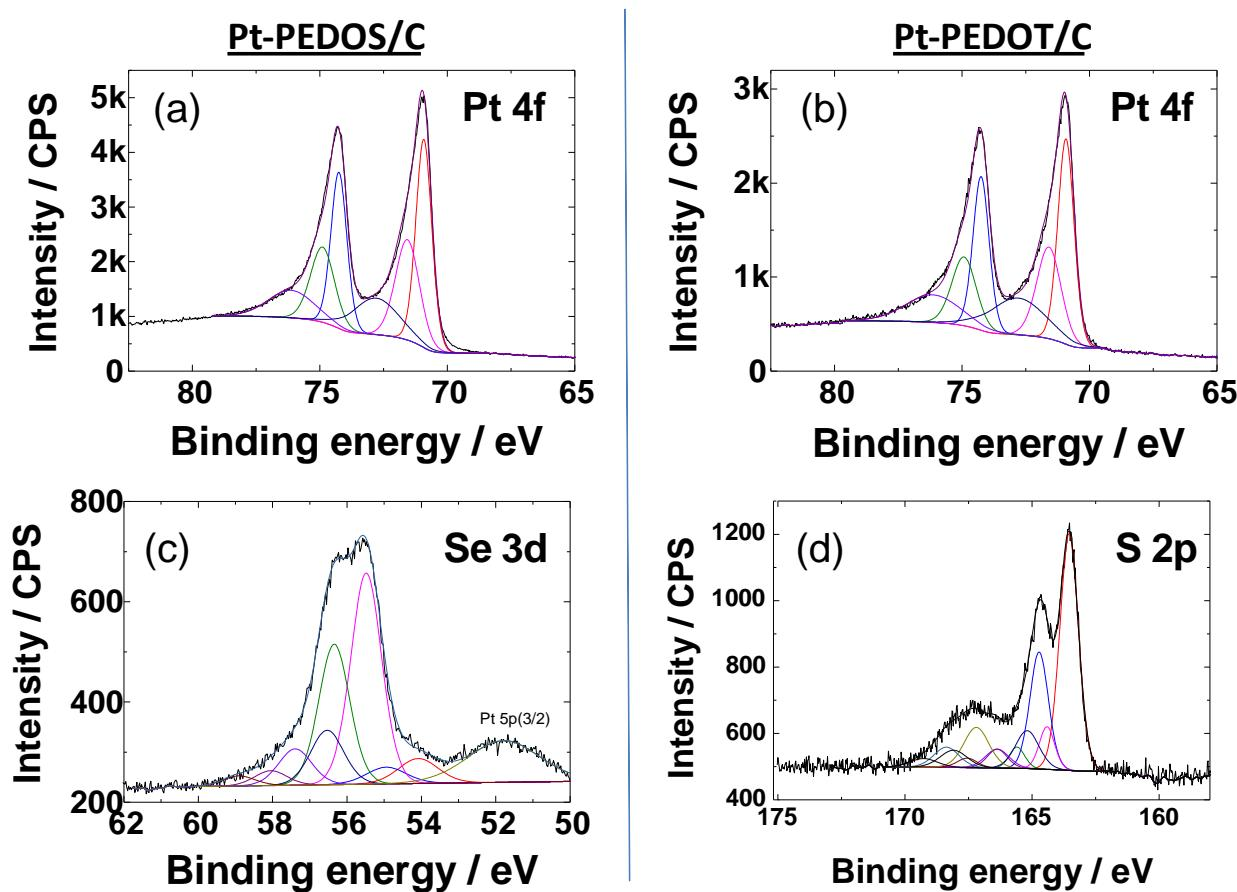
**Figure S1.** High resolution XPS of (a) the Pt 4f region of Pt-PEDOS/C, (b) the Pt 4f region of Pt-PEDOT/C electrode, (c) the Se 3d region of Pt-PEDOS/C electrode, and (d) the S 2p region of Pt-PEDOT/C electrode.
