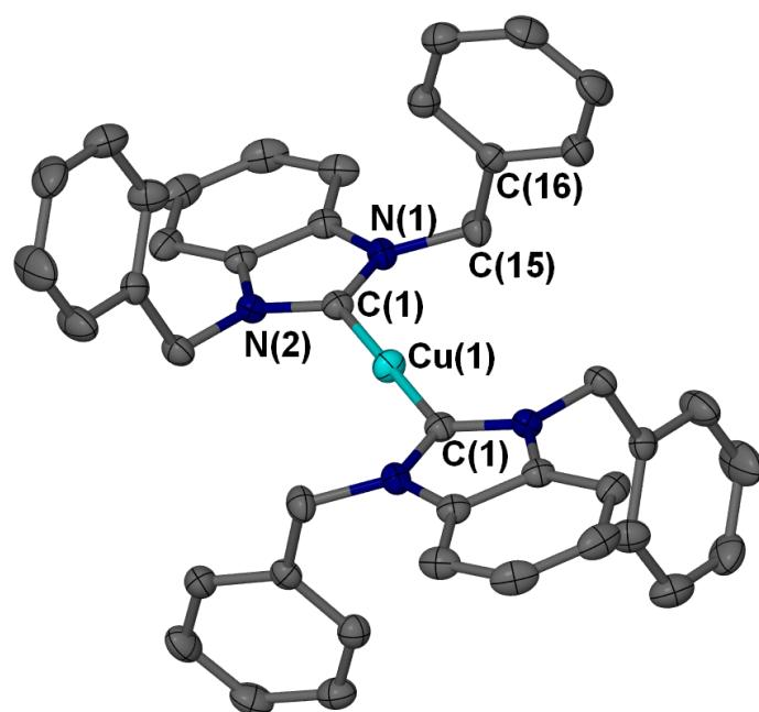
**Figure S3** Solid-state structure of **5d**. Selected bond distances ( $\text{\AA}$ ) and lengths (deg): C(1)-Cu(1) 1.9066(15), C(1)-N(1) 1.3523(19), C(1)-Cu(1)-C(1) 180.00(7), N(1)-C(1)-Cu(1) 126.41(11), C(16)-C(15)-C(1) 112.98(12).
