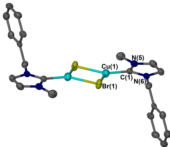
**Figure S4** Solid-state structure of **6c**. Selected bond distances (Å) and lengths (deg): C(1)-Cu(1) 1.932(6), Cu(1)-Br(1) 2.4506(13), C(1)-N(6) 1.363(7), C(1)-Cu(1)-Br(1) 127.94(18), Cu(1)-C(1)-N(6) 126.2(4), N(6)-C(5)-C(6) 112.8(4).
