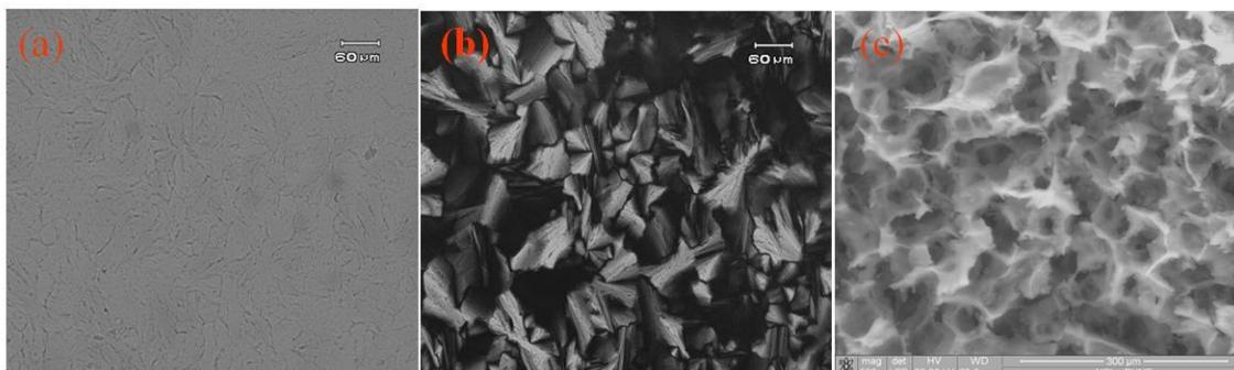
**Figure SI 4:** Optical micrographs and SEM images of Scaffold obtained by one pot synthesis. (a) Corresponding optical micrograph under parallel polarizers showing the phase separated mesoporous silica particles forming a network at the boundaries of the birefringent domains. (b) Corresponding crossed optical microscope image (showing birefringence due to different domains of the H1 phase). (c) SEM of the scaffold obtained by one pot synthesis.
