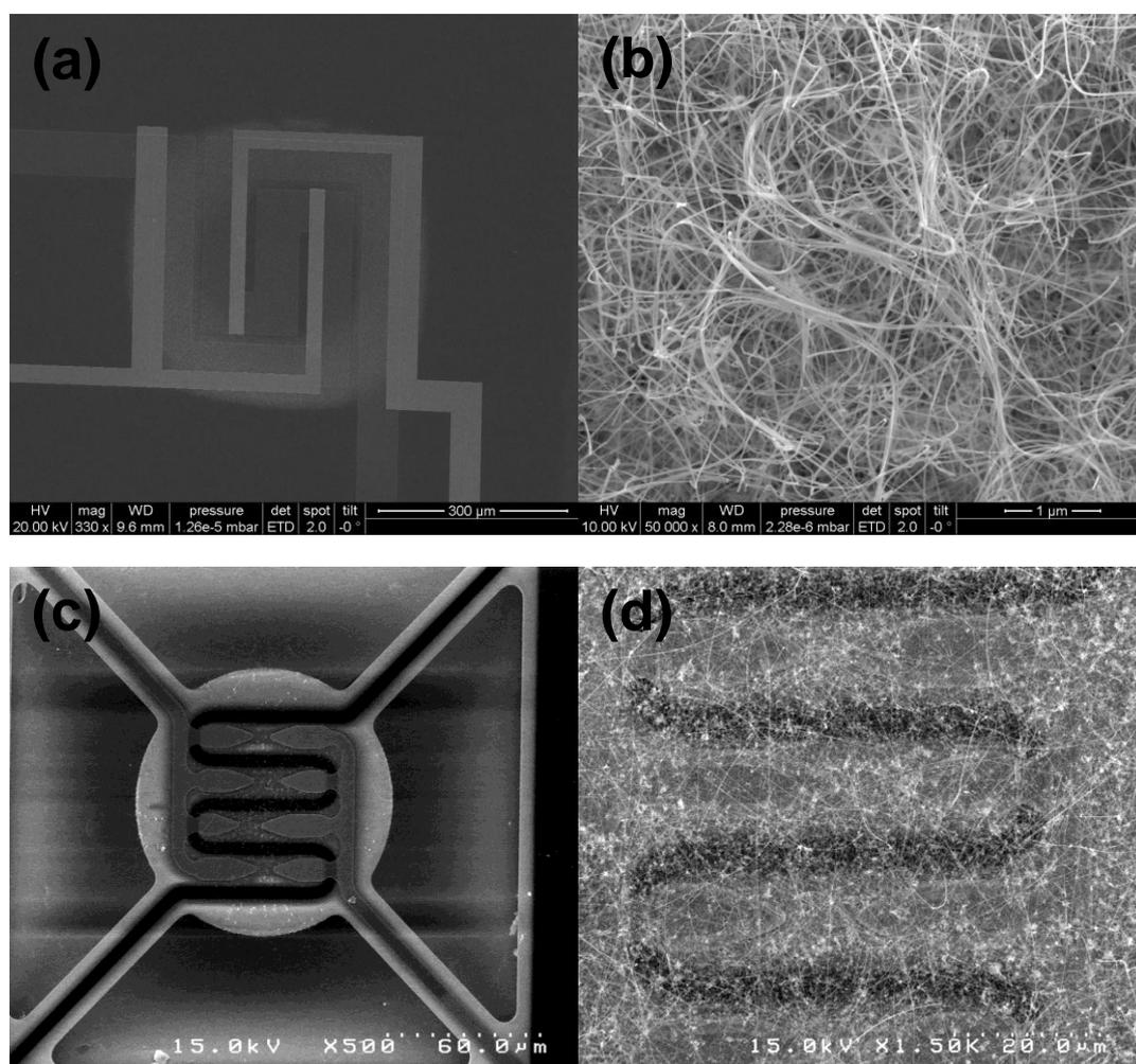
**Fig. S1** (a) Site-selective growth of Ge NWs using micro-membranes and (b) SEM image of the homogeneous Ge nanowire coating. (c) and (d) show similar deposits on free-standing micro-hotplates at ~400 °C with low coverage in the centre and ~450 °C higher magnification of dense nanowire bundles at higher temperature, respectively.
