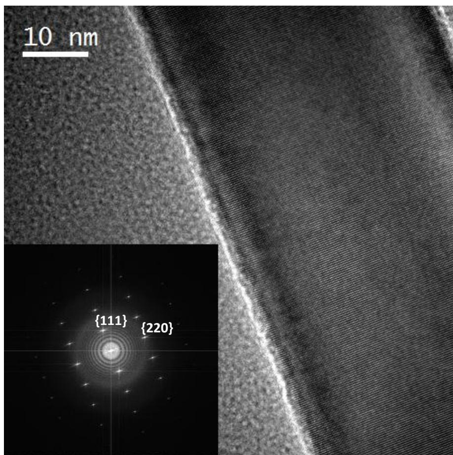
**Fig. S2** HRTEM of a  $\langle 111 \rangle$ -oriented Ge nanowire grown on a micro-membrane illustrating the excellent crystal quality of the germanium nanowire, which is also reflected in the sharp FFT (inset).
