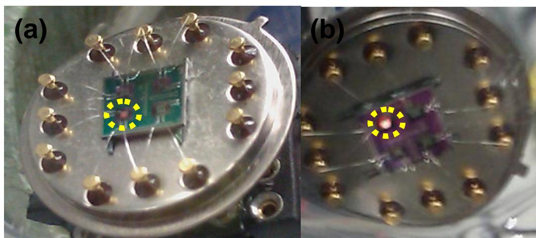
**Fig. S3** Photographs of a micro-membranes heated to 700 °C in a glass chamber. The heated area is glowing due to the high temperature and indicated by yellow circles to guide the eye. Distortions in the image are due to the non-planar shape of the glass chamber used to visualize this effect.
