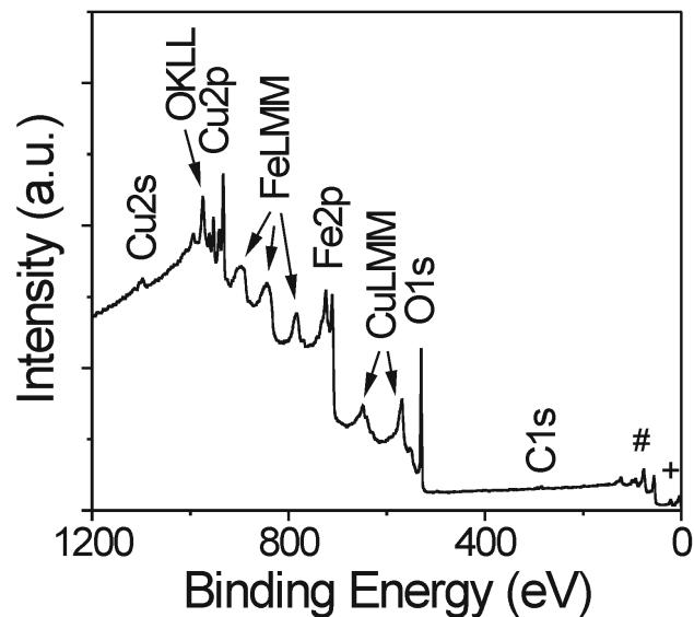
**Figure S6.** XPS survey spectrum of a ~175 nm thick, KLE-templated  $\text{CuFe}_2\text{O}_4$  spinel film heated to 650 °C in air. The  $\text{Cu}3\text{s}/\text{Fe}3\text{s}/\text{Cu}3\text{p}/\text{Fe}3\text{p}$  and  $\text{O}2\text{s}$  core level regions are indicated by (#) and (+), respectively. Apart from a very weak carbon C1s peak, which we associate with adventitious hydrocarbon at the top surface, only copper, iron, and oxygen core levels are observed.
