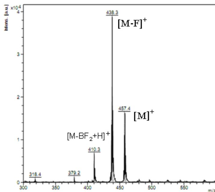
**Figure S5.** MALDI-TOF –MS spectrum of **2**.
