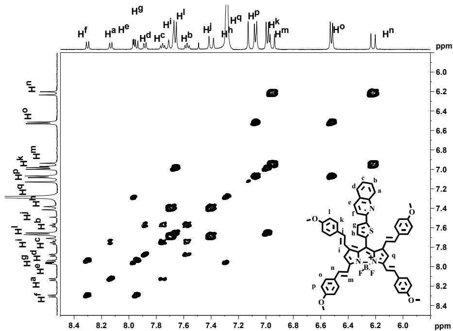
**Figure S7.**  $^1\text{H}$ - $^1\text{H}$  COSY spectrum of **1**.
