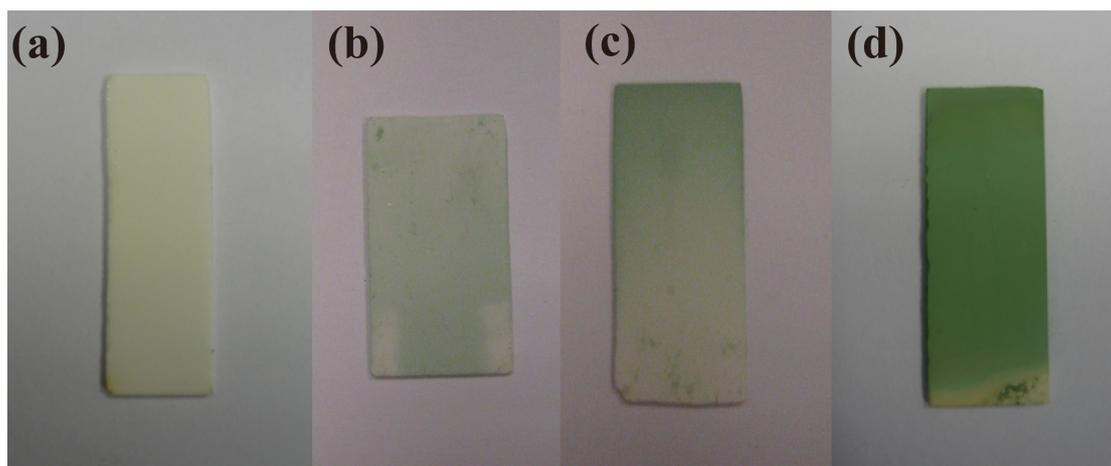
**Fig. S1.** Digital photographs of (a) alumina plate, (b) MIL-101(Cr) film synthesised via the 'reactive seeding' method, (c) MIL-101(Cr) synthesised without DMA wetting on the alumina plate and (d) MIL-101(Cr)-A film synthesised with DMA wetting on the alumina plate.
