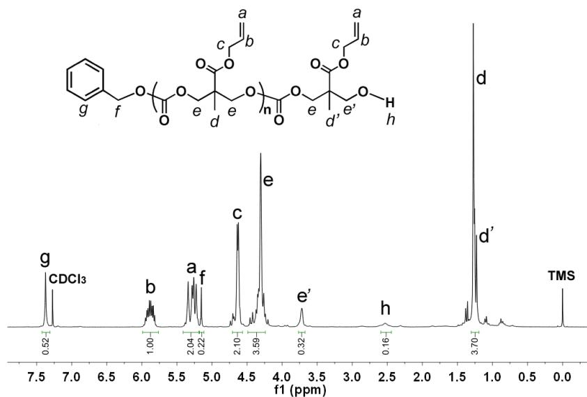
**Figure S2.** <sup>1</sup>H NMR (300MHz, CDCl<sub>3</sub>, 25 °C) spectrum of PMAC. Conditions: [MAC]<sub>0</sub> = 0.33 M, [MAC]<sub>0</sub>:[BnOH]<sub>0</sub>:[Lu]<sub>0</sub> = 100:10:1, THF, 100% conversion,  $T_p$  = 25 °C.
