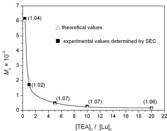
**Figure S1.** Dependence of the molar mass  $M_n$  (PDI indicated in parentheses) on  $[TEA]_0/[Lu]_0$  ratio. Conditions: [MAC]<sub>0</sub>-to-[Lu]<sub>0</sub> ratio = 100, [MAC]<sub>0</sub> = 0.33M, Solvent, THF,  $T_p$  = 25 °C.
