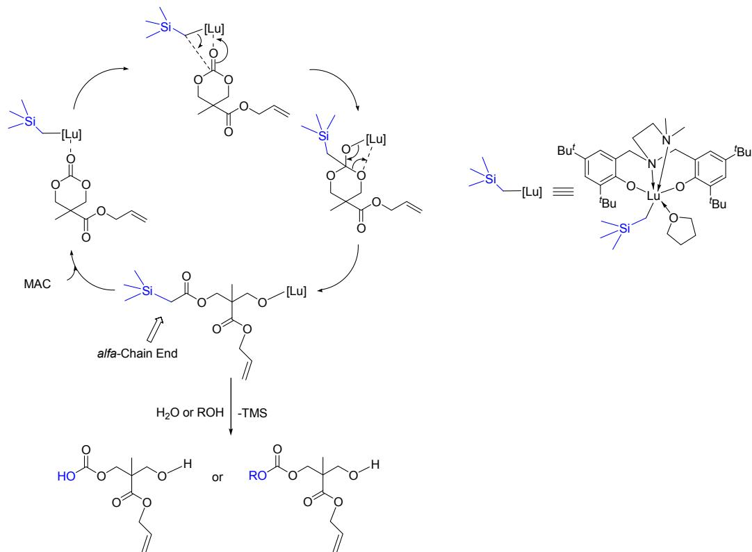
**Figure S5.** Coordination-insertion mechanism for the ROP of MAC using complex **1** in absence of alcohols.
