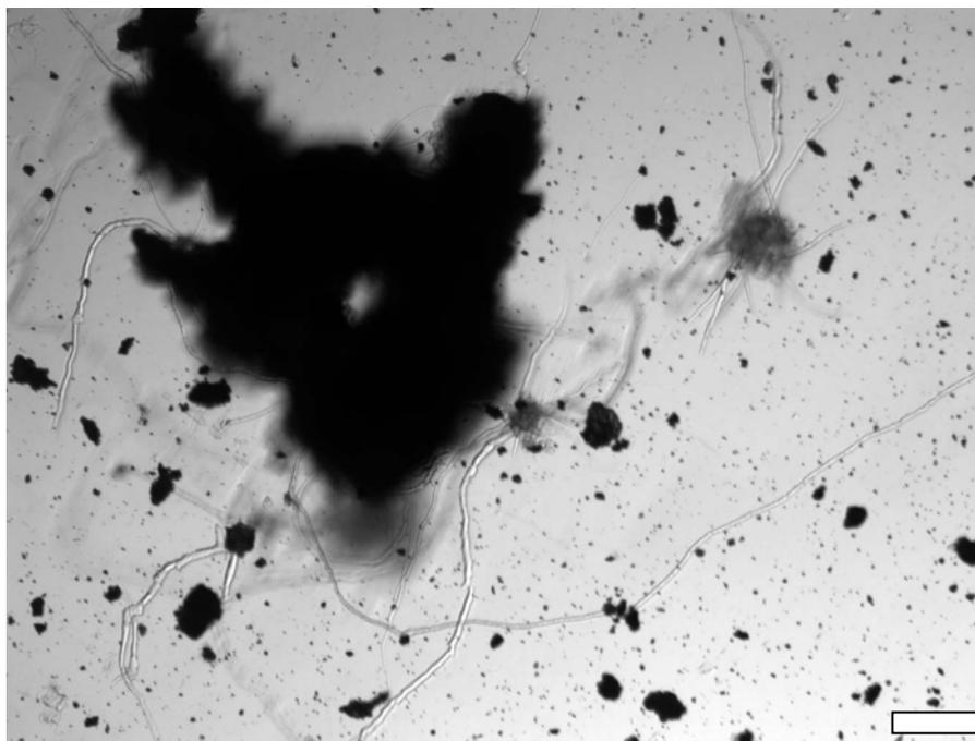
**Fig. S8:** Dissolution of a pellet made of 1:1  $(\text{C}_4\text{H}_{10}\text{NO})_{40}[\text{W}_{72}\text{Mn}_{12}\text{O}_{268}\text{Si}_7].48\text{H}_2\text{O}$ .  $4(\text{C}_4\text{H}_9\text{NO})$  (B):Starch in a solution of Me-DIP Br (concentration  $2 \times 10^{-2}$  mol/L). Scalebar is 50  $\mu\text{m}$  long.
