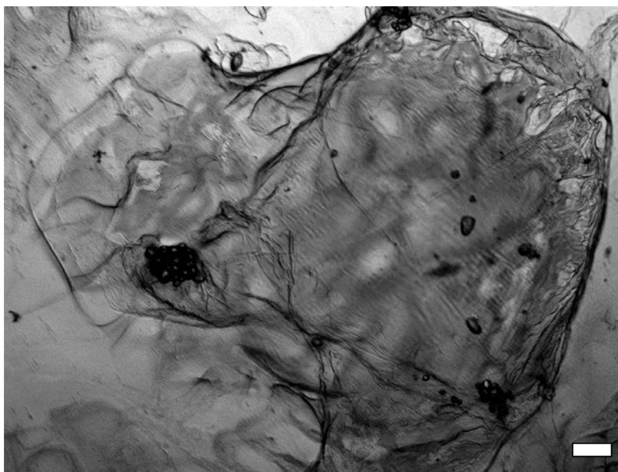
**Fig. S2:** Dissolution of a pellet made of pure Phosphotungstic acid (D) into a solution of Me-DIP Br (concentration  $2 \times 10^{-2}$  mol/L). Scalebar is 100  $\mu$ m long.
