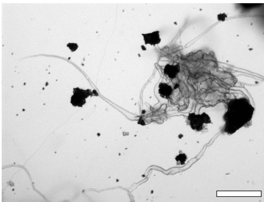
**Fig. S12:** Dissolution of a pellet made of 1:1  $(\text{C}_4\text{H}_{10}\text{NO})_{40}[\text{W}_{72}\text{Mn}_{12}\text{O}_{268}\text{Si}_7].48\text{H}_2\text{O}. 4(\text{C}_4\text{H}_9\text{NO})$  (B):Starch in a solution of Me-DIP Br (concentration  $2 \times 10^{-2}$  mol/L), using ground crystals as the POM precursor. Scalebar is 100  $\mu\text{m}$  long.
