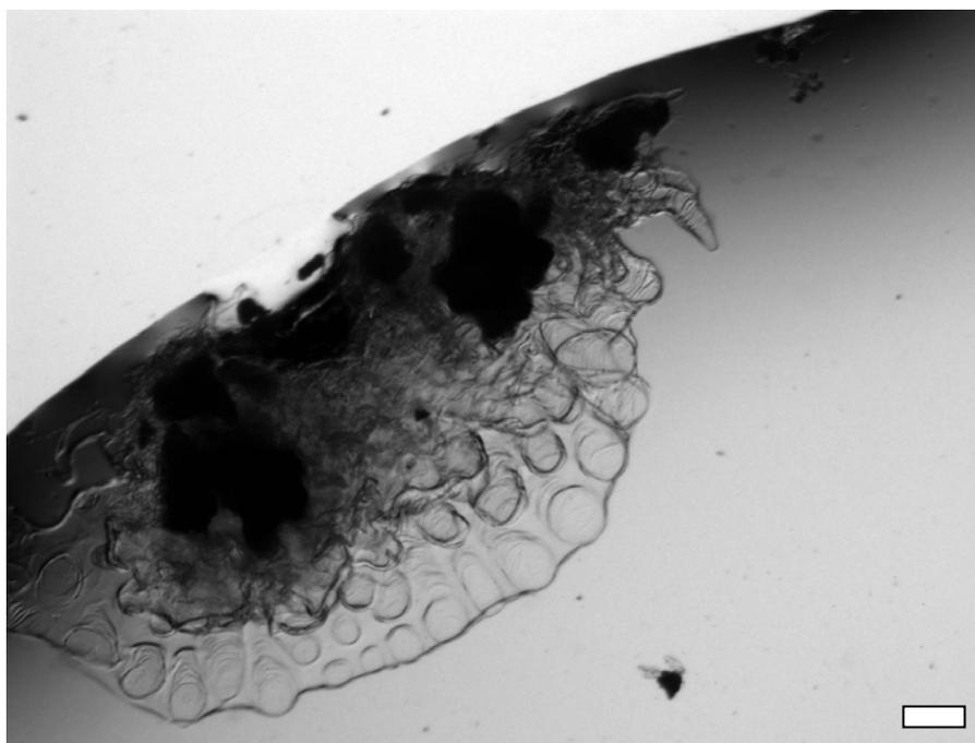
**Fig. S4:** Dissolution of a pellet made of 1:1 Phosphotungstic acid (**D**): *tert*-butylammonium in pure water. Membrane formation highlights the non-innocence of TBA towards tube growth. Scalebar is 100  $\mu$ m long.
