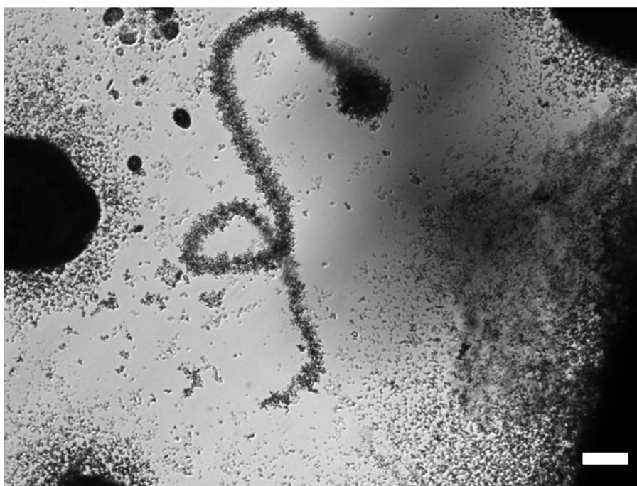
**Fig. S9:** Dissolution of a pellet made of 1:2  $\text{Na}_{15}[(\text{PO}_2)_3\text{PNb}_9\text{O}_{34}]$  (C):Starch in a solution of Me-DIP Br (concentration  $2 \times 10^{-2}$  mol/L). Scalebar is 50  $\mu\text{m}$  long.
