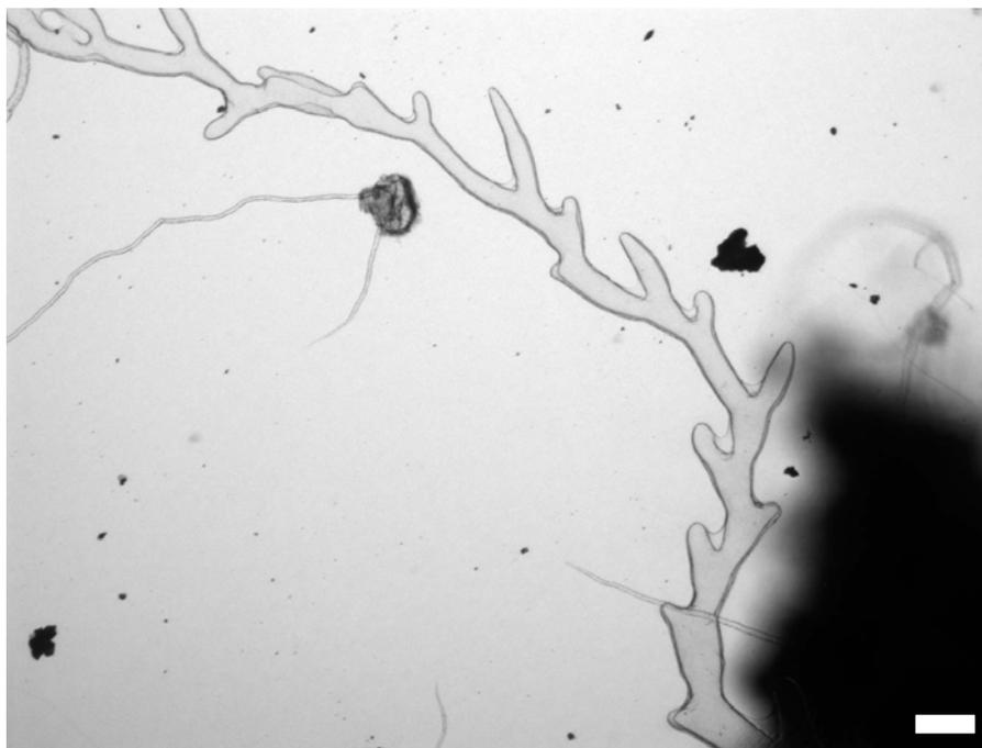
**Fig. S3:** Dissolution of a pellet made of 1:1 Phosphotungstic acid (**D**):*tert*-butylammonium into a solution of Me-DIP Br (concentration  $2 \times 10^{-2}$  mol/L). Scalebar is 100  $\mu$ m long.
