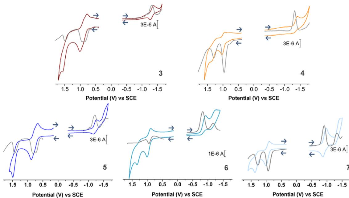
**Figure S2:** Cyclic Voltammogram and DPV results of **3-7** in DCM.
