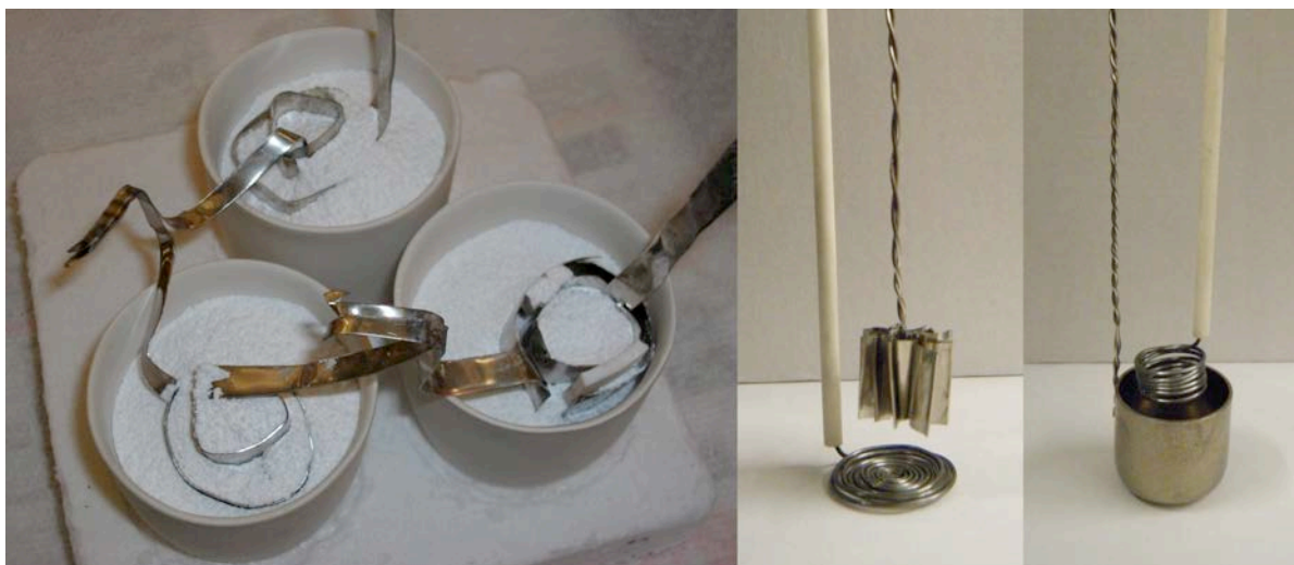
Figure 3. Configurations and components used in the STEP electrolysis experiments. Left side: three electrolyses in series, with lithium carbonate using thin planar nickel and steel electrodes, prior to the melt, and prior to addition of external insulation. Middle: high surface area nickel electrode prepared by folding a single rectangle of pure nickel (25 \mu\text{m} or 75 \mu\text{m} thick), connected by spot welded nickel wire (99.5%. 1.0 mm) situated above a cathode for carbon deposition prepared by coiling steel wire, and is shown prior to insertion in the alumina crucible and prior to carbonate addition. Gas evolved from the central electrode can be directed with a large circumference alumina tube (not shown). Right side, high temperature configuration: coiled steel wire cathode in a nickel crucible, which acts both as the cell case and the anode, and is shown prior to the addition of the internal carbonate and external insulation.
