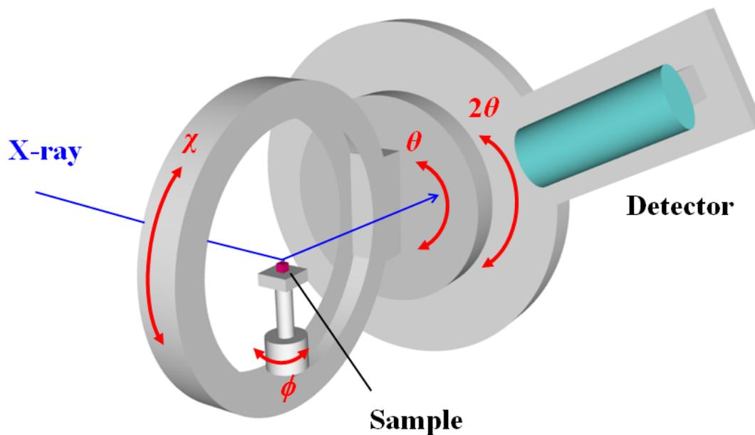
**Fig. S3** The schematic drawing of the four-circle diffractometer at beamline BL13XU for surface and interface structures, SPring-8.
